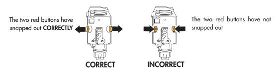
Check that the two red buttons have snapped out, otherwise the door cannot be closed.
