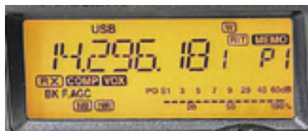
Figure 5 — The IC-7200's amber display is small but very readable. It includes indicators for often-used features and settings.
