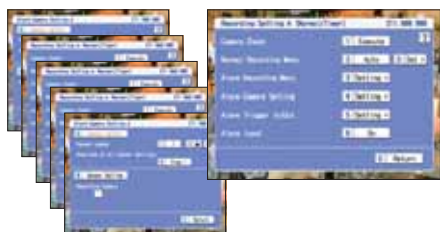
Set recording parameters separately for each camera
