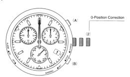
When performing the all-reset procedure, first make sure that the watch is fully charged and the second hand is moving in one second increments. If the allreset procedure is performed when the watch is insufficiently charged, it may not function properly or remain stopped following the all-reset procedure.
