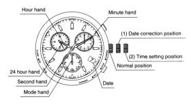
2. When the crown is pulled out to Position 2 (time setting position), the second hand rapidly advances to the 0 position and stops.
