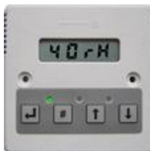
To enter the software menu for setup mode, hold the **Enter** and **Down** buttons together for approximately 3 seconds until the message "Ent" appears on the display. Release both buttons and now press the Enter button again to enter the software menu. IO is the first item to be displayed. Scroll up or down to go through the menu items which are highlighted below.
