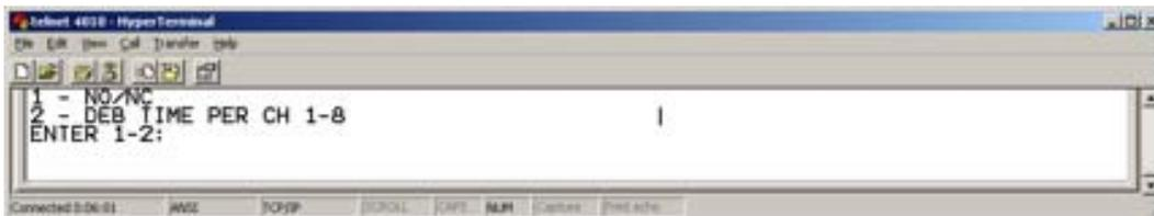
When 1 is selected from the menu: Make changes or press **ESC**ape to accept current values. If changes are made, all eight values must be entered in sequence.
