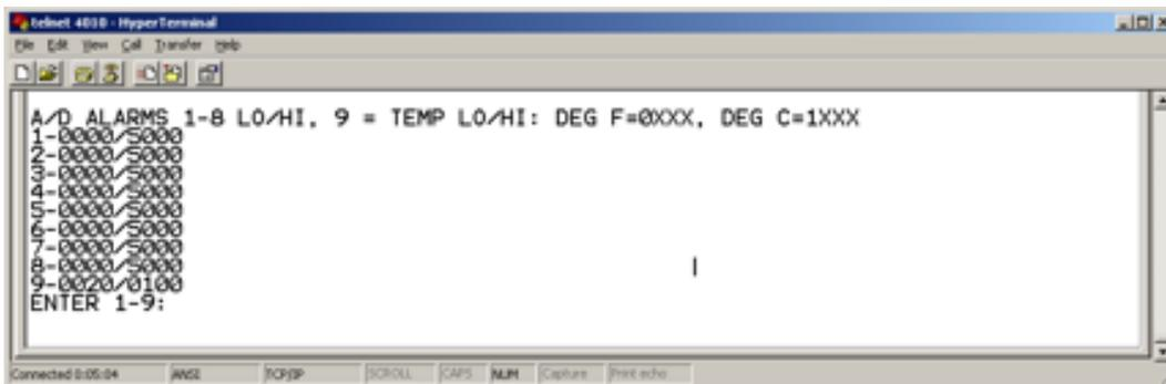
When “6” is selected from the PGM menu, the Status inputs are set up for either Normally Open or Normally Closed and the required **DE**Bounce time needed before generating an alarm.
