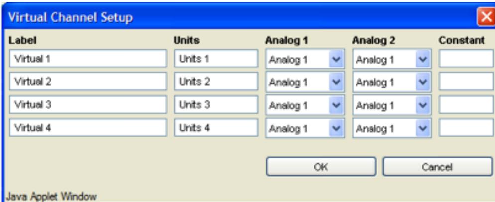
The WVRC-8 lets you define up to four “virtual” channels. These are similar to analog channels, but their values are derived from the product of two real analog channels and a constant.
