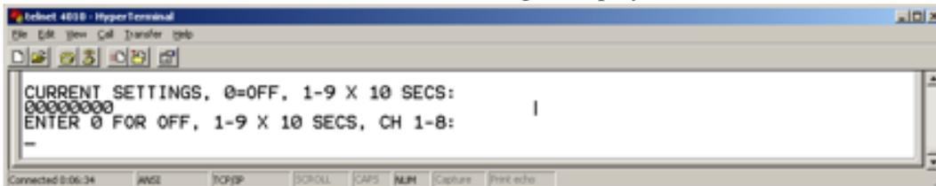
Make changes or press **ESC** to accept current values. If changes are made, all eight values must be entered in sequence. Valid settings are 0 through 9. A “0” will turn off the status input so that it will not generate an alarm. Entering any number from 1-9 will set the “DEBounce” period from 10 to 90 seconds, requiring the input to be in an alarm state for that amount of time before an alarm is generated. Any interruption will cause the timer to reset.
