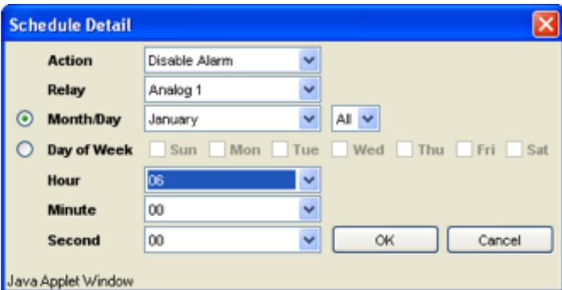
The Schedule Detail Dialog is used to set up a single schedule event. An event specifies an action (raise or lower), a relay or alarm muting/unmuting, and a time when the action occurs. The scheduler supports both day-of-month and day-of-week schedules. Wildcards can be specified in any of the date/time fields to create a repeating event.
