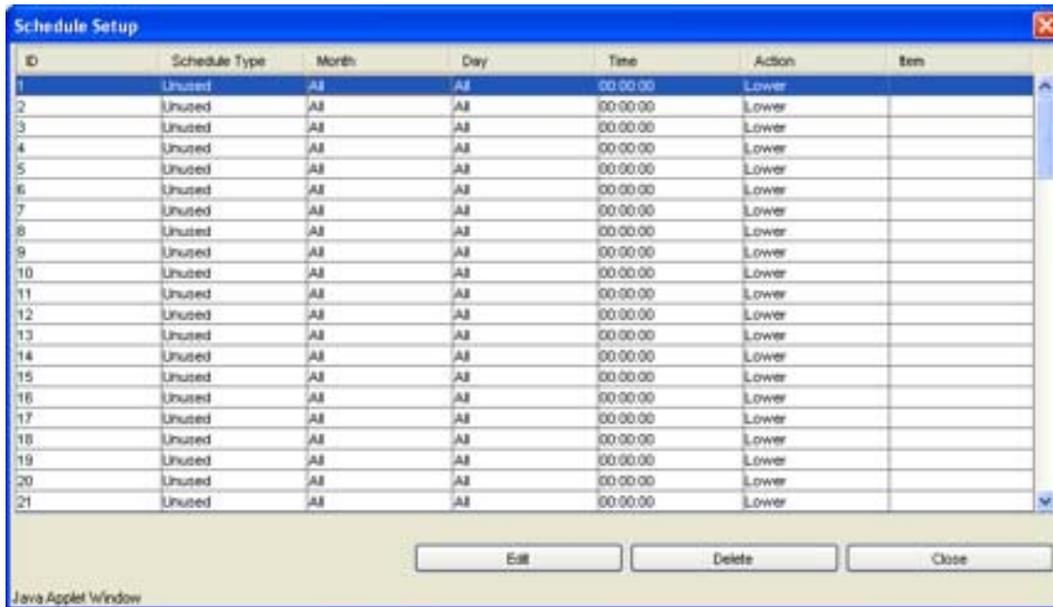
Raise, lower relays and alarm enable/disable can be activated on a scheduled basis. Up to 100 scheduled events can be defined. These can be one-time or repeating events. The Schedule Setup Dialog displays a list of scheduled events and allows the user to edit the schedule event's details, described under Schedule Detail Dialog below.
