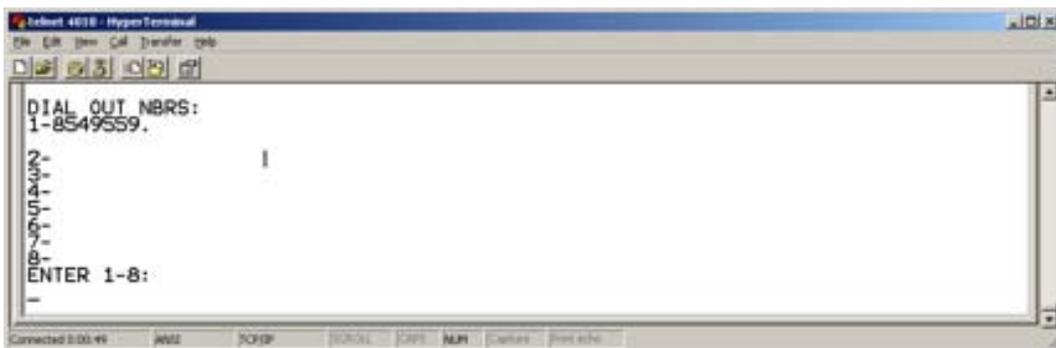
These are the numbers that will be dialed when alarms are generated. The dial-out list will select numbers from this pool to call out during an alarm condition. Up to 32 digits can be used in each number along with a comma (,) for one second and a semi-colon (;) for 5 second pauses.
