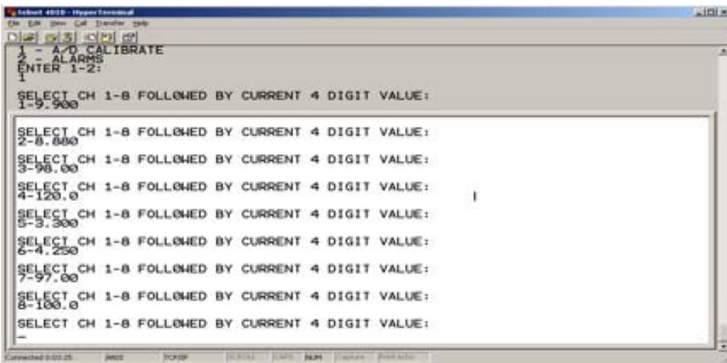
Enter a “2” from the Analog Set-Up menu to establish alarm set points. Analog (metering) input set points are set up using items 1 - 8, representing analog (metering) inputs one thru eight.
