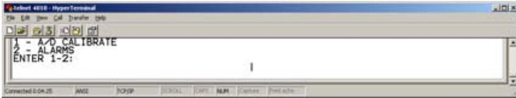
Select “1” to calibrate any of the analog (metering) inputs for the desired value. Selecting a “1” will produce the following prompt “Select Ch 1-8 followed by the desired 4 digit value”. Enter the channel number, then the desired value.
