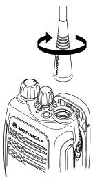
1 Turn the antenna clockwise to attach it.
