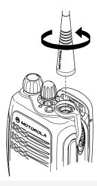
Turn the antenna counterclockwise to remove it.
