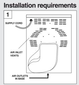
**IMPORTANT:** This dryer must be installed such that the air inlets and outlets are not restricted (fig. 1).
