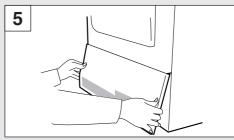
2. Pull firmly on the handgrip and slide the water container out of the dryer (fig. 6).
