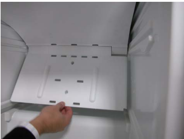
l) Cut the air diffuser pulling and lifting it up.
