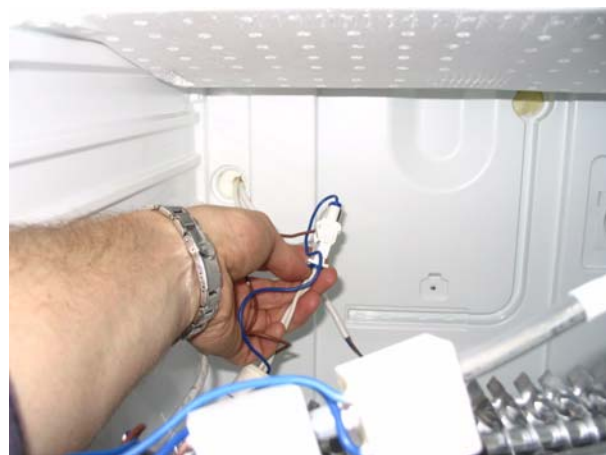
u) Unplug the connector of the thermal switches.
