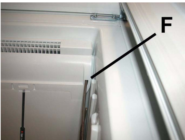
f) Insert a blade inside the F slot and release the internal hook.
