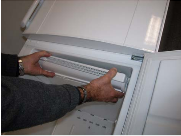
h) Lift and pull the air vent grid.
