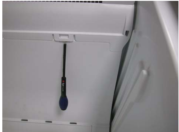
e) Insert a screwdriver into the right hook and release it.
