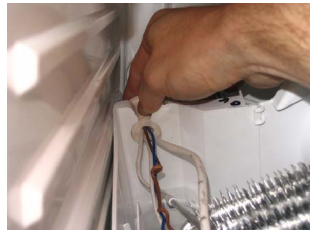
s) Remove the sealing rubber.
