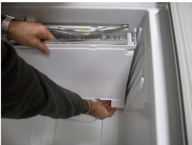
n) Pull backward the cold module support releasing the rear water drain duct.
