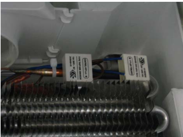
r) Cut the wiring tie of the thermal switches and release them from the evaporator. Note: The defrosting and cut-out thermal switches (+8 / +40°C) are connected together, therefore they are not available as single spare parts.
