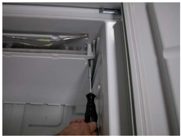
m) Remove the 2 fixing screws of the cold module.
