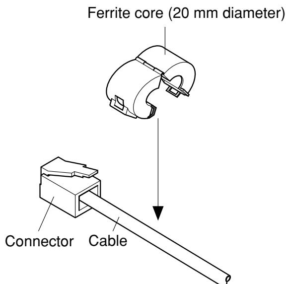
Pass the fastener through the ferrite core.
