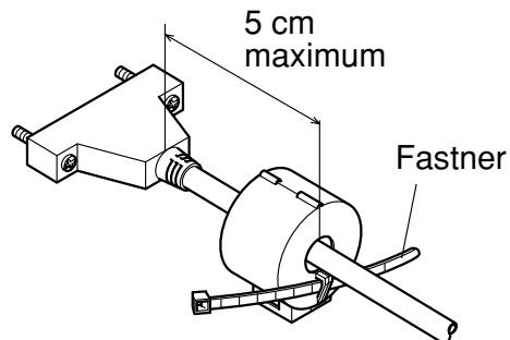
Loop the fastener around the cable and lock it. Use scissors to cut off any excess.
