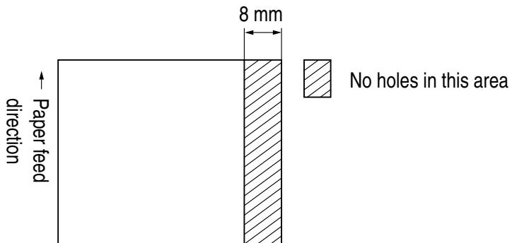
Do not use paper with perforations within the shaded area. Perforations may cause the paper sensor to erroneously report an out of paper condition.
