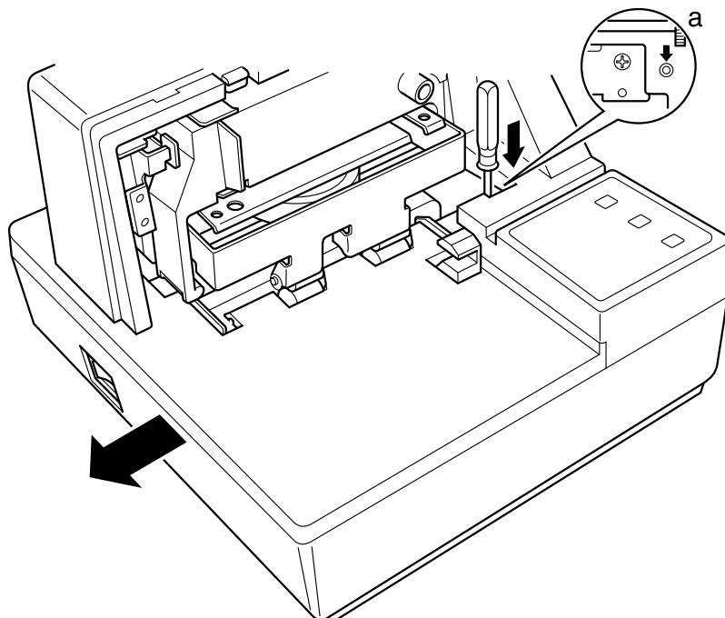
It is not necessary to remove the document table completely, just move it enough so you can get at the DIP switches inside.
