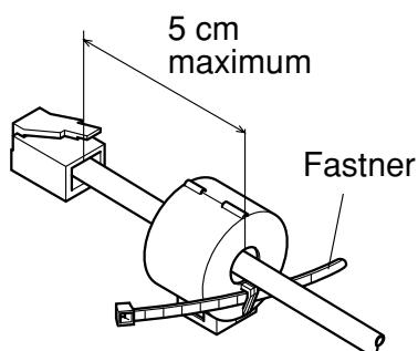
Loop the fastener around the cable and lock it. Use scissors to cut off any excess.
