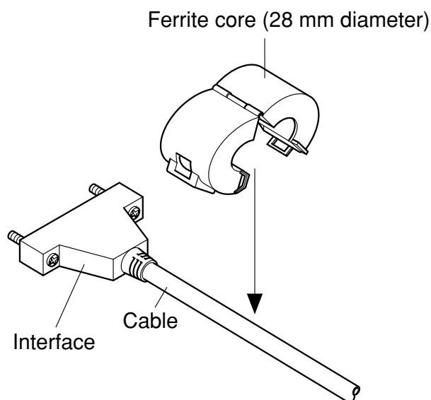
Pass the fastener through the ferrite core.
