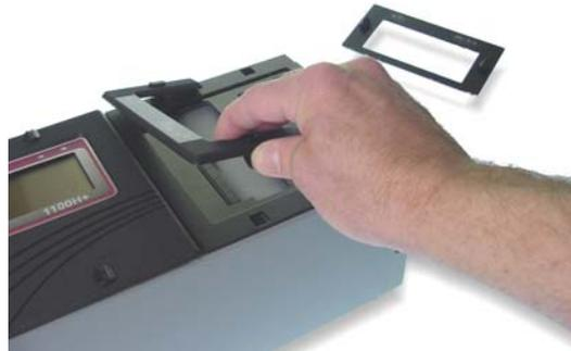
4. Remove and set the scanner assembly next to the tester.
