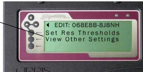
6. Set the desired value for the Test Parameter Setting. When selected, some Test Parameter Settings toggle between two values. Others scroll to the desired value.
