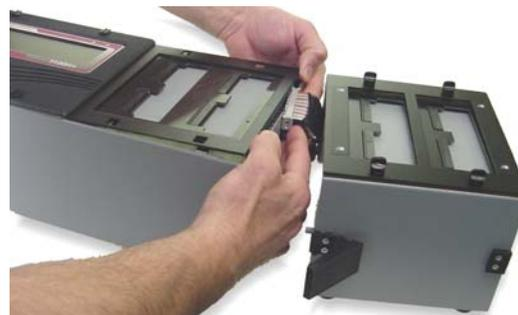
9. Attach the Scanner Add-On to the base tester using the side latches.
