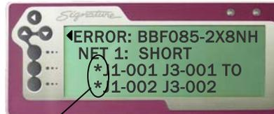
Asterisks are added to the pins in the net that are closest to the short. The tester does this using resistance measurements.
