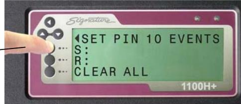
The S event sets (or sinks) the output pin to ground thereby allowing current to flow through the output circuit.
