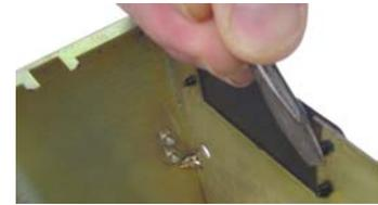
**To remove the plastic rivets holding the cover piece, use a screwdriver or any hard flat object to push in the rivet plunger, then remove the plunger.**
