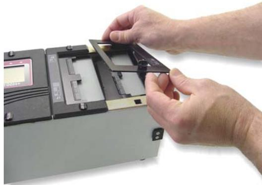
3. Slide in an adapter until it is fully seated.
