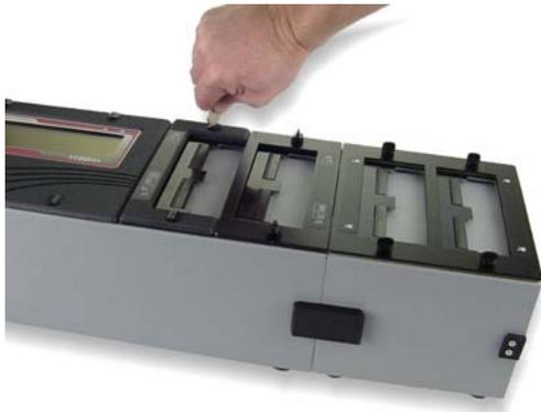
11. Use a permanent marker to write the adapter positions on each add-on cover plate.
