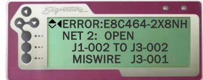
As shown in this example, the miswire error is always indicated as a contact OPEN to where it should go, and MISWIRE to where it does go.
