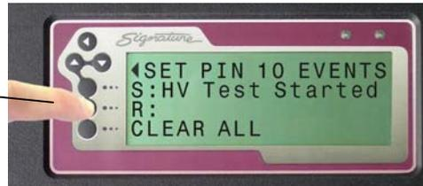
The R event resets the output pin to the original no current flowing state.
