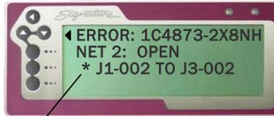
An asterisk is added to the pin closest to the open. The tester can do this by sensing the lower capacitance of the unconnected pin.
