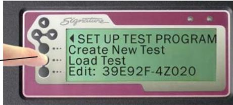
3. Scroll to the memory location containing the test.
