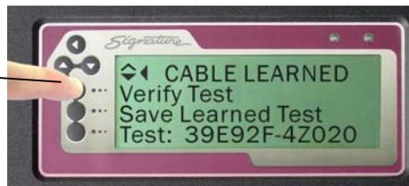
If you are storing the cable to a memory location, make sure to write the location down on the *1100R+ Cable Documentation*, or on the *1100R+ Memory Location Listing* (blank in the appendix). For more information see *Using the Tester Memory* on page 19.
