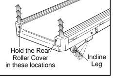
back end, first raise it past the highest position, and then lower it. CAUTION: Before exercising, push on the back of the treadmill to make sure that the incline legs are locked in position. Do not place objects under the treadmill to change the incline; change the incline only as described above.
