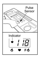
your thumb slightly until the heart-shaped indicator in the Calories/Fat Calories display flashes steadily. Hold your thumb at this level. After 5 to 10 seconds, your pulse will be shown. Hold your thumb on the pulse sensor for another 15 seconds for the most accurate reading.
