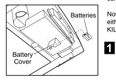
into the battery compartment. Make sure that the negative ends of the batteries (marked "-") are touching the springs. Close the battery cover.
