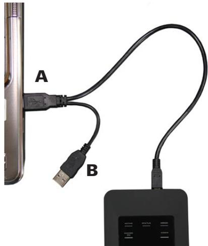
**Note:** Do not use the DIGITTRADE HIGH SECURITY HDD via a bus-powered USB hub or USB extension cable.
