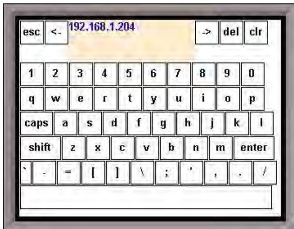
This option will allow the user to modify the IP address of the *9120 Instrument* only. The address must be supplied in a 999.999.999.999 format, or it will not be accepted. Contact Super Systems at 800-666-4330 or your IT department before changing any of the IP addresses.
