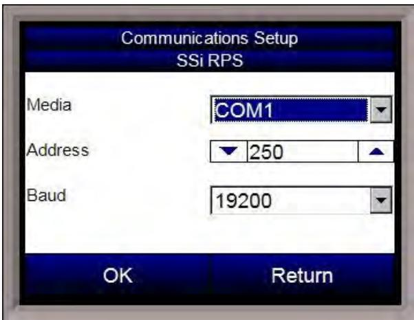
The communications setup screen will allow the user to configure how the touch screen will communicate with the 9120 instrument. The "Media" drop-down list will set the communications media (COM ports or Ethernet). The options are: **COM1, COM2, COM3, COM4, or Ethernet.**
