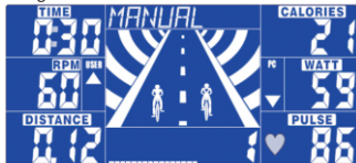
Workout in Manual mode, user may set up value and start workout, console will count down to 0.
