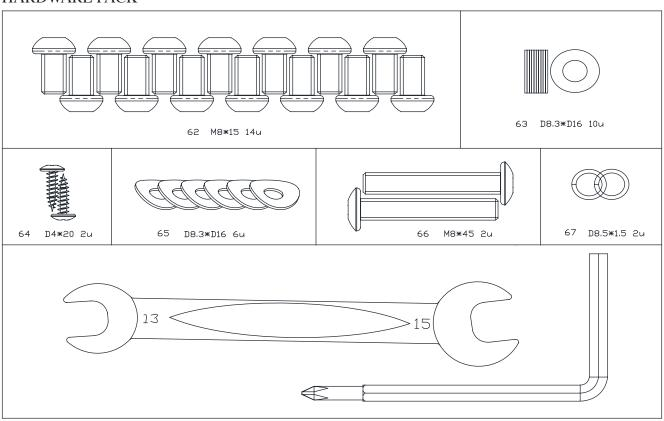
Attach the Front Stabilizer (31) to the frame, then secure it with Allen screw (62) and Flat washer (63) tightly. Use the same step to assemble the Rear Stabilizer (48).
