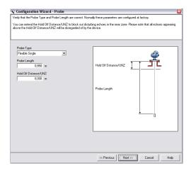
Verify that the parameters in the *Probe* window are correct. The
