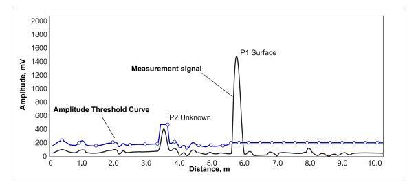
Figure 6-4. Disturbing echoes can be filtered out by registration as False Echoes
