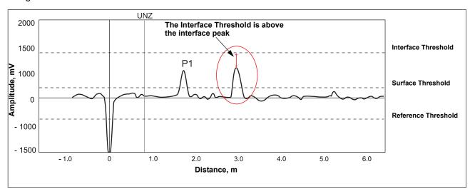
If the Interface Threshold is too high, the signal amplitude peak at the interface between the upper and lower products is not detected.
