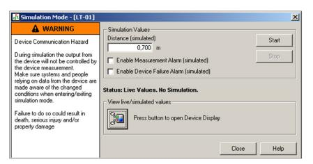
Also, or alternatively, activate the transmitter's loop test function. Output 4, 12, and 20 mA and verify that the readings in the DCS match up.
