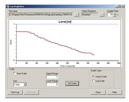
Start emptying the tank or chamber making sure not to stop until it is completely empty. With a chamber, do not forget to close the process valves before draining.
