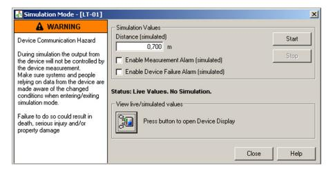
Also, or alternatively, activate the transmitter's loop test function. Output 4, 12, and 20 mA and verify that the readings in the DCS match up.
