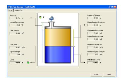
Figure 3-7. Presentation of Analog Output value in Rosemount Radar Master
