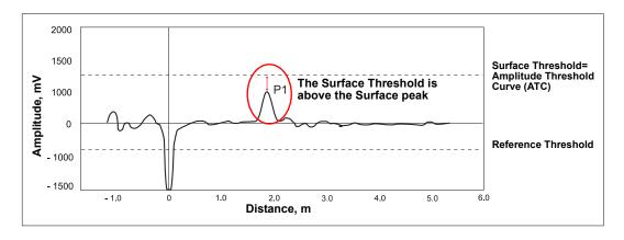
Figure 4-7. Surface threshold is too low
