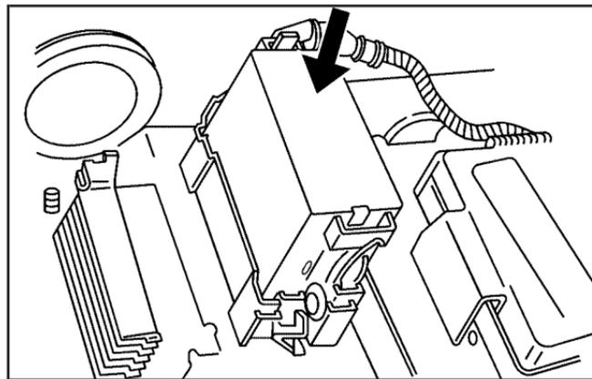
4. Locate the relay center inside the box. It is located toward the driver's side of the vehicle.
