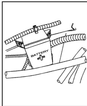
The remote positive (+) terminal is located inside a red cover in the engine compartment on the passenger's side of the vehicle. See item A in the *Engine Compartment Overview on page 5-12*.
