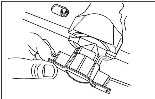
1. Remove the cover of the housing located behind the license plate area by pushing in the tabs and pulling downward.
