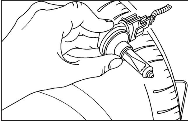
5. Disconnect the bulb socket from the wiring harness and replace the unit.
