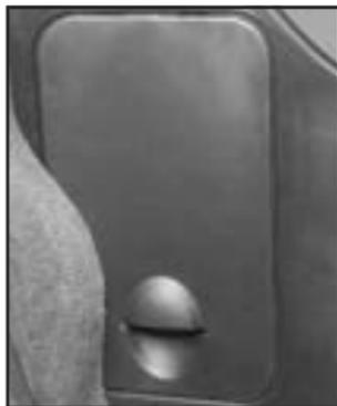
The floor console fuse block is located on the console between the two seats, on the passenger's side.
