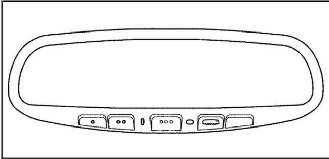
If your vehicle has this feature, the Universal Home Remote transmitter buttons are located on the automatic dimming rearview mirror. The three buttons on the left side of the mirror are the Universal Home Remote transmitter buttons.
