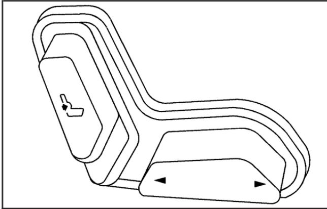
The power seat controls are located on the outboard side of the passenger's seat.
