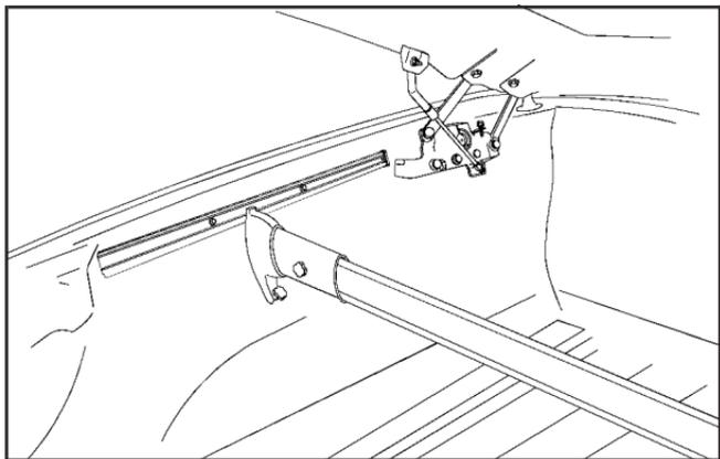
5. Position the cross bar vertically between the side rails as shown.
