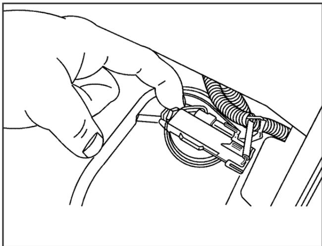
2. Remove the socket from the lamp assembly by locating and then squeezing the release tab while turning the socket counterclockwise.
