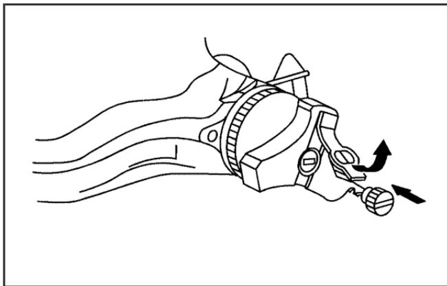
2. Hold the ball rod tight with one hand, tighten the handwheel slightly and turn it clockwise as far as it will go.
