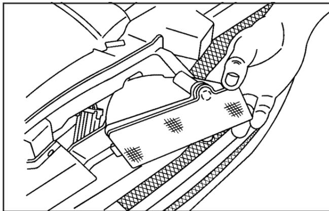
5. Locate and release the tabs behind the grille that hold the lamp assembly in place. Unsnap the tabs and push forward to remove the lamp assembly.
