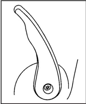
To fold the seatback forward, push the lever on the side of the seatback rearward and pull the seatback forward.
