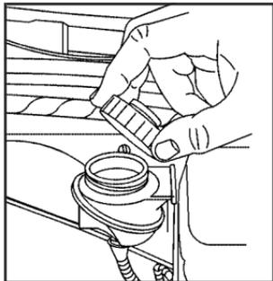
Refer to the Maintenance Schedule to determine how often you should check the fluid level in your master cylinder reservoir and for the proper fluid. See *Owner Checks and Services on page 6-8* and *Recommended Fluids and Lubricants on page 6-12*.
