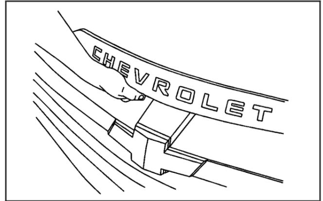
2. Release the secondary latch at the front of the hood.
