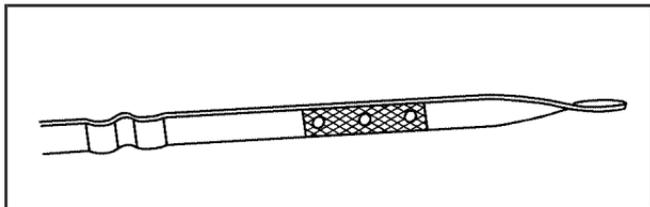
If the oil is below the cross-hatched area at the tip of the dipstick, you will need to add at least one quart/liter of oil. But you must use the right kind. This section explains what kind of oil to use. For engine oil crankcase capacity, see *Capacities and Specifications on page 5-95*.
