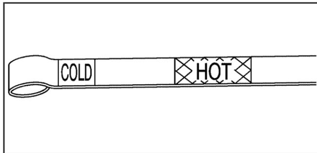
3. Check both sides of the dipstick, and read the lower level. The fluid level must be in the COLD area, below the cross-hatched area, for a cold check or in the HOT or cross-hatched area for a hot check. Be sure to keep the dipstick pointed down to get an accurate reading.
