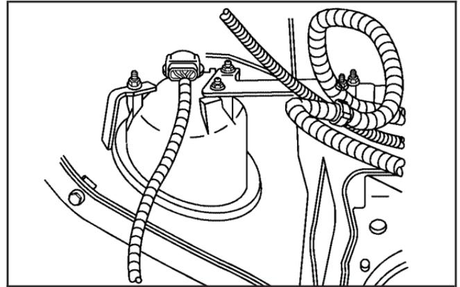
2. Find the bulb socket, twist counterclockwise, and remove it from the lamp assembly.
