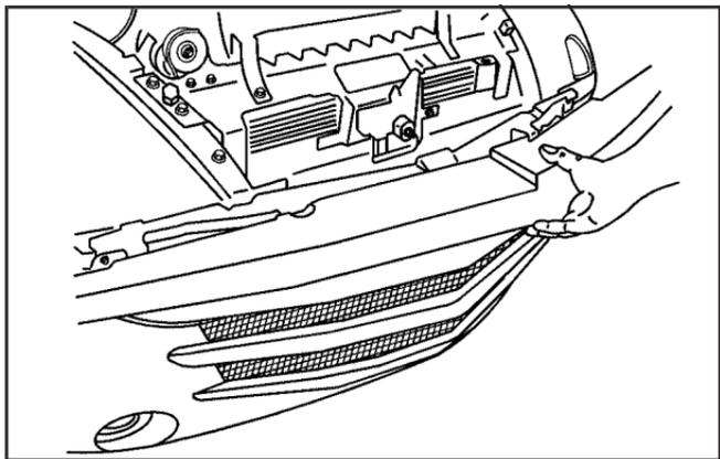
4. Pull outward on the bar to remove it from the vehicle.
