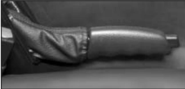
To set the parking brake, hold the brake pedal down. Pull the parking brake lever up. If the ignition is on, the brake system warning light will come on. See *Brake System Warning Light* on page 3-30 for more information.
