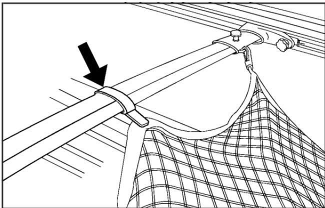
15. Wrap the hook and loop strap around the cross bar as shown to secure the middle portion of the cargo net.
