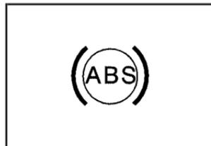
If there is a problem with the anti-lock brake system, this warning light will stay on. See *Anti-Lock Brake System Warning Light* on page 3-31.
