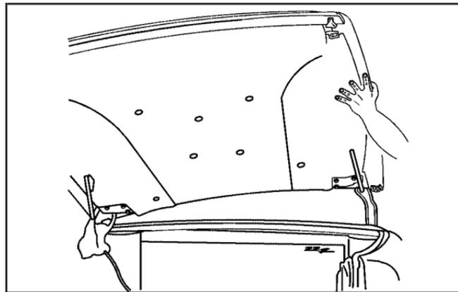
4. Slide the cover rearward and then lift up on the passenger's side of the cargo cover. Then have another person lift the driver's side of the cargo cover.
