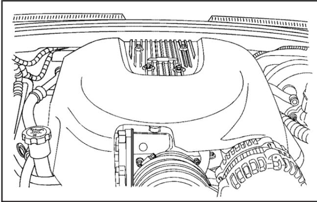
1. Unscrew the four bolts from the engine.
