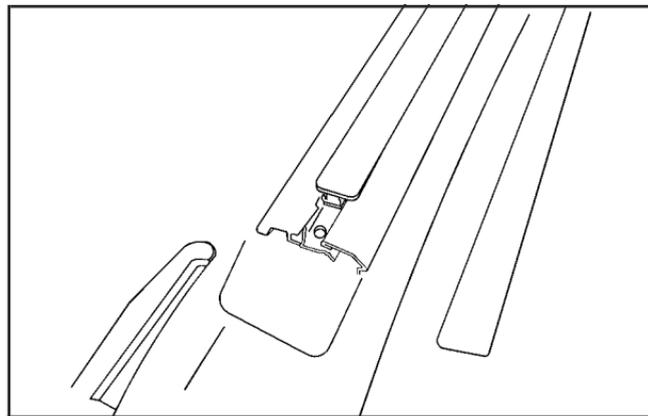
4. Insert the cover into the floor track and slide it all the way forward.
