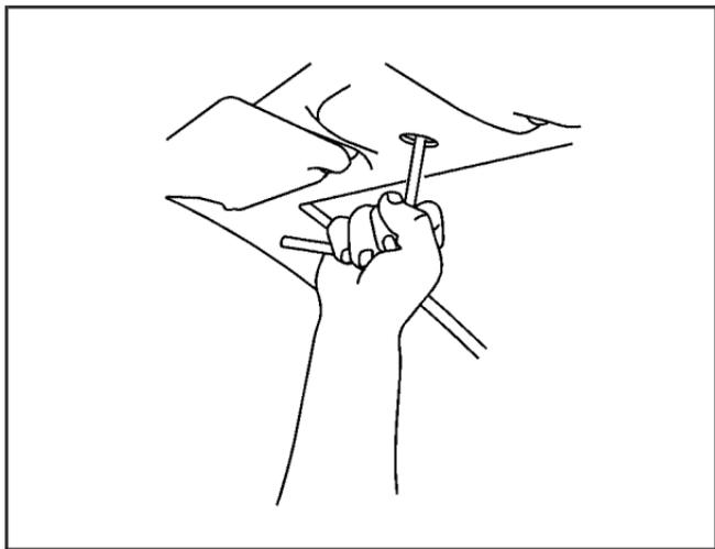
13. Insert the convertible top release tool into the latch closing mechanism between the sun visors and turn it counterclockwise until the latches are secured and the convertible top is fully closed.
