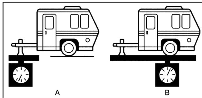
The trailer tongue weight (A) should be 10 percent to 15 percent of the total loaded trailer weight (B), up to a maximum of 250 lbs (113 kg) with the equipped hitch.
