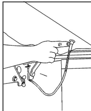
2. Disconnect the electrical connector located on the underside of the cargo cover near the front of the bed, if equipped.
