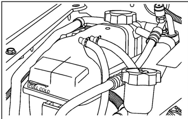
The engine coolant surge tank is located on the passenger's side of the vehicle at the rear of the engine compartment. See *Engine Compartment Overview* on page 5-12 for more information on location.
