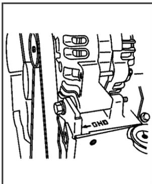
The remote negative (-) terminal is located near the power steering fluid reservoir. It is marked GND (-). See item H in the *Engine Compartment Overview* on page 5-12 for more information on location.
