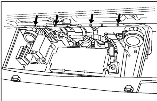
2. Locate the water-tight box that houses the relay center and remove the four nuts that secure the cover to the backside of the passenger compartment.
