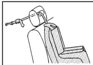
If the position you are using has a halo head restraint and you are using a single tether, route the tether through the hole in the head restraint.
