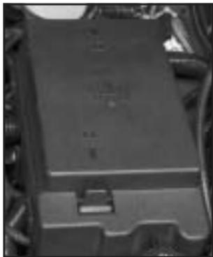
The fuse block is located under the hood in the engine compartment on the driver's side of the vehicle. See *Engine Compartment Overview* on page 5-12 for more information on location.
