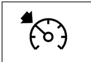
The cruise light on the instrument panel cluster will illuminate when the cruise control is engaged.
