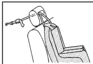
If the position you are using has a halo head restraint and you are using a dual tether, route the tether through the hole in the head restraint.
