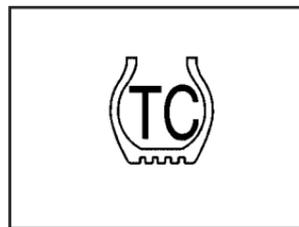
To turn the system on or off, press the traction control button located on your center console switchbank. See *Center Console Switchbank* on page 3-19 for more information.
