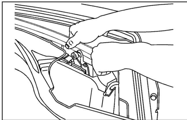
9. Grasp the front panel of the convertible top and pull up.
