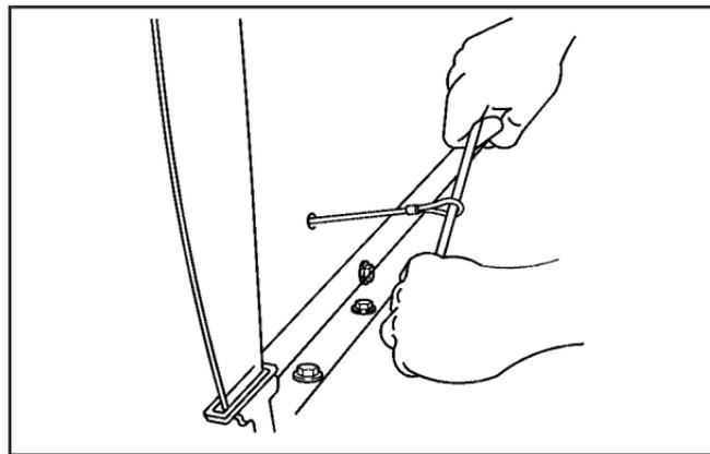
6. Pull the cable with the release tool.
