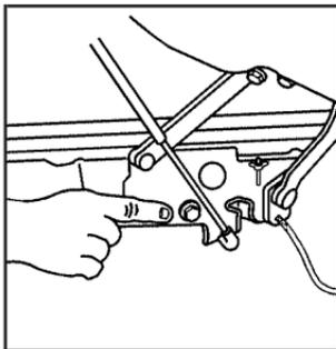
3. Locate and remove the bolts that hold the cargo cover in place. There is one bolt on each side near the front of the cargo area.
