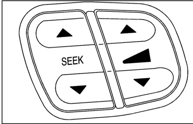
Some audio controls can be adjusted at the steering wheel. They include the following:
