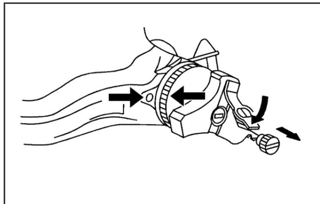
1. Open the lock cover on the handwheel and unlock with the key.
