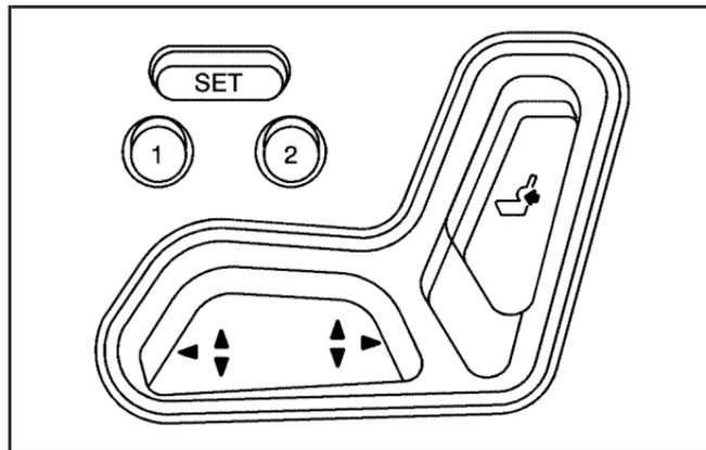
Your vehicle may have a memory driver's seat. The controls for this feature are located on the outboard side of the driver's seat and are used to program and recall memory settings for the driver's seating positions.
