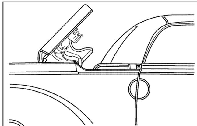
1. Open the convertible top until the roof tonneau and the boot cover panel are upright so that you can reach into the convertible top storage area as shown. See *Lowering the Convertible Top on page 2-47* for more information.
