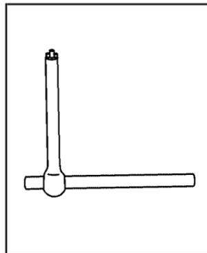
12. Slide the tool side of the convertible release tool until the entire tool forms a right angle as shown.
