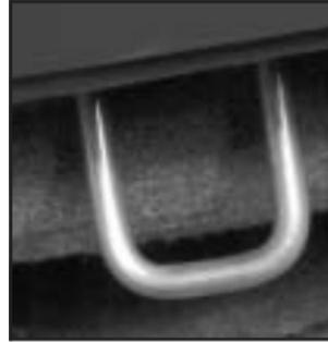
The top tether anchor is located on the back of the front passenger seat.
