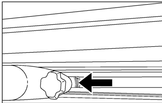
8. Slide the locking tabs in the side rails until they are aligned with the knobs on the cross bar as shown and loosely tighten the knobs.
