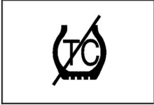
If the TC (traction control) warning light comes on and stays on, there may be a problem with the traction control system.
