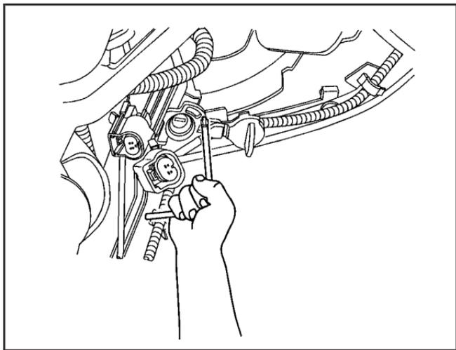
2. Insert the convertible top release tool and turn it to activate the emergency release. The convertible top release tool is provided by the dealer and stored in the glovebox. See your dealer if the convertible top release tool is misplaced.
