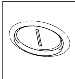
11. Remove the plastic cap located between the sun visors by turning it one quarter turn.
