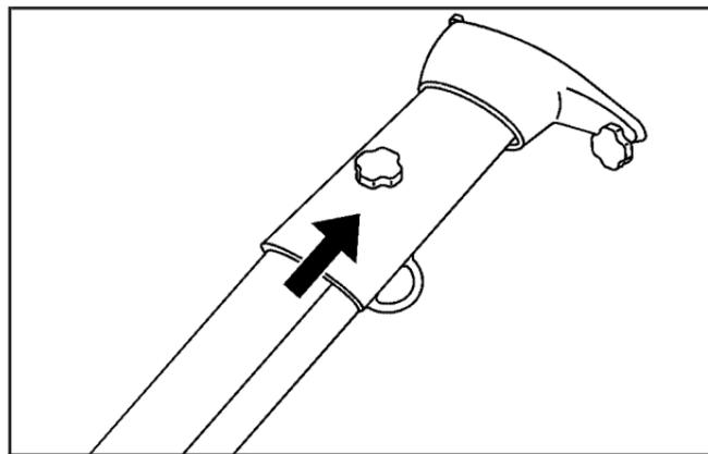
4. Loosen the knobs located on top of the telescoping cross bar by turning them counterclockwise.
