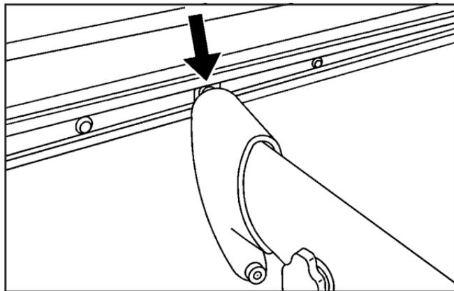
6. Insert the tabs located at each end of the cross bar into the side rails.
