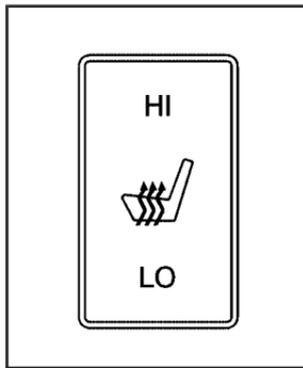
If your vehicle has this feature, the switches are located on the outboard side of the driver's and passenger's seats.
