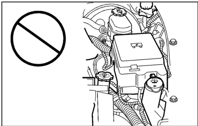
**Notice:** Jump starting your vehicle's battery using the engine compartment fuse block battery posts can damage your vehicle. See item K in the *Engine Compartment Overview on page 5-12*. Always use the remote positive terminal and remote negative terminal to jump start your vehicle's battery. See items A and H in the *Engine Compartment Overview on page 5-12* for location.
