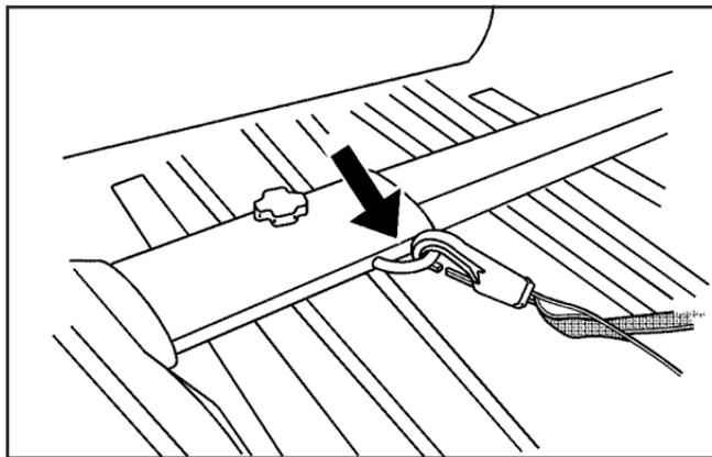
14. Clip the other end of the cargo net to the telescoping cross bar as shown.
