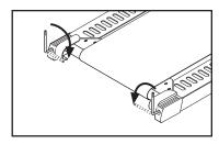
ment bolt counterclockwise, 1/4 of a turn each. Be careful not to overtighten the walking belt. Walk on the treadmill for a few minutes. Repeat until the walking belt is centred.
