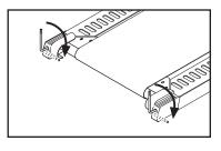
the walking belt is correctly tightened, you should be able to lift each side of the walking belt 5 to 7 cm (2 to 3 in.). Walk on the treadmill for a few minutes. Repeat until the walking belt is properly tightened. Be careful to keep the walking belt centred.
