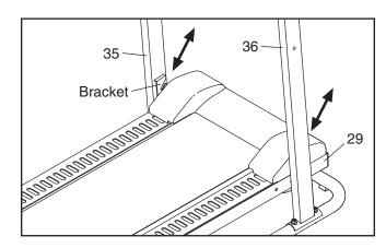
**A CAUTION:** Make sure that the incline knobs are fully inserted at the same height.
