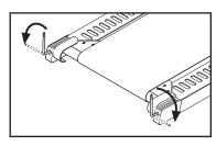
adjustment bolt clockwise, 1/4 of a turn each. Be careful not to overtighten the walking belt. Walk on the treadmill for a few minutes. Repeat until the walking belt is centred.
