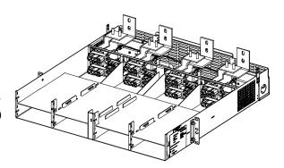
♦ The 8-position Module Mounting Shelf is equipped with individual Rectifier Module (PCU) AC input feeds (one branch circuit per module mounting position, eight feeds total).
