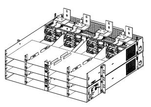
Each 8-position Module Mounting Shelf in the assembly is equipped with individual Rectifier Module (PCU) AC input feeds (one branch circuit per module mounting position, eight feeds total per shelf, sixteen feeds total per assembly).
