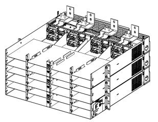
♦ Each 8-position Module Mounting Shelf in the assembly is equipped with individual Rectifier Module (PCU) AC input feeds (one branch circuit per module mounting position, eight feeds total per shelf, twenty-four feeds total per assembly).
