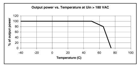
Warning: The module is rated for continuous operation at full output power up to +50°C (+122°F). Operation between +50°C (+122°F) and +65°C (149°F) will result in output power decreasing by approximately 33 Watts/°C. Operation above +65°C (+149°F) is considered abnormal and should be used on a temporary¹ basis only.
