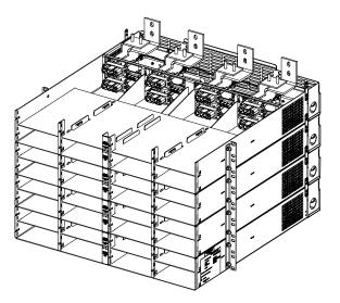
♦ Each 8-position Module Mounting Shelf in the assembly is equipped with individual Rectifier Module (PCU) AC input feeds (one branch circuit per module mounting position, eight feeds total per shelf, thirty-two feeds total per assembly).
