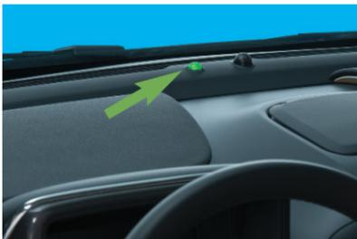
**Note:** Immediately after plugging in, the charging status indicator may be amber for up to five seconds before turning green. The charging system may run fans and pumps when the vehicle is turned off.
