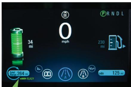
The Total Range indicator displays the total distance that can be driven, based on the combined electric and extended range, before recharging or refueling the vehicle.
