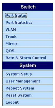
The function menus contain two parts: **Switch** for setting up the switch functions and **System** for maintaining the system parameters.
