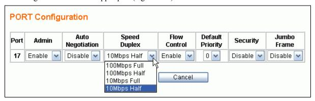
NOTE: Only full duplex mode is supported in 1Gbps link speed. <u>For copper medium, this system doesn't support 1Gbps link speed in force mode</u>; for fiber medium, only the 1Gbps link speed is supported, but either auto or force mode can be set to build up the link.
