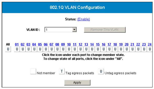
The following figure shows the **802.1Q VLAN Port Configuration** page by port. (e.g. Port10)
