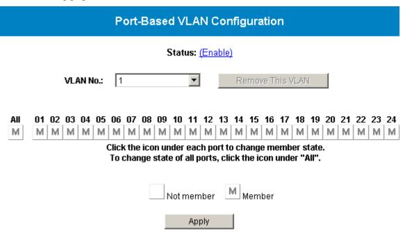
You can add, delete, and modify the port-based VLAN for your need. Currently this system supports **up to 32** port-based VLAN groups for manual entry. The next pages will be described in detail how to configure the port-based VLAN.
