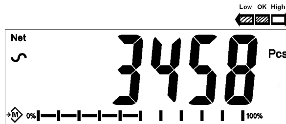
Checkweighing during Parts Counting
