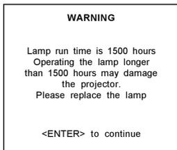
*Lamp run time is 1500 hours. Operating the lamp longer than 1500 hours may damage the projector. Please replace the lamp.*
