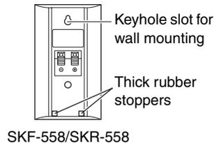
To mount the center speaker horizontally, use the two keyhole slots shown to hang the speaker on two screws that are securely screwed into the wall.
