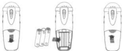
(Diagram #1) - Installing the batteries
