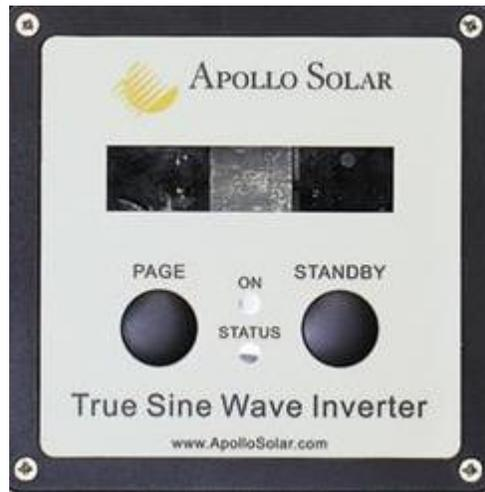
Figure 1.0: TSW Control Panel
