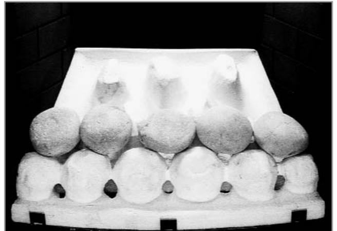
3. Take five more ceramic pebbles and position as shown to form the 'second row' of the fuel effect. The pebbles may be rotated as desired to fit into the gaps between the supports in order to create a random, realistic effect. Again, remember not to push the pebbles down too far into the valleys between the supports as this can have a detrimental effect to the flame picture.
