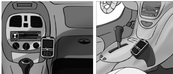
Figure 13: Main unit installation.
