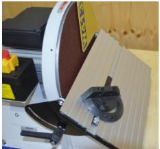
There is a scale on the trunnion, for accurate angle setting of the table.
