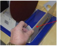
Swing the top of the dust collection hood forward and lift it clear of the base.
