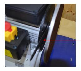
Should it ever be necessary to remove the disc, the motor spindle can be locked with the largest of the three spanners provided and the disc unscrewed. It has a standard right hand thread.
