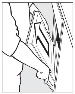
Hold the door securely at both sides and lift upwards off the hinge guides.
