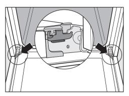
Before removing the door, the locking clamps on both hinges have to be released.
