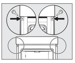
Open the oven door and using two screws secure it to the side walls of the housing unit through the holes in the oven trim.
