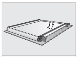
Refit the glass fibre seal.
