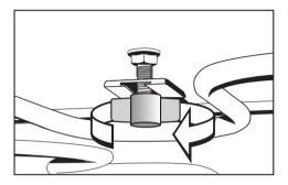
Unscrew the wing nut and lower the top heating element.
