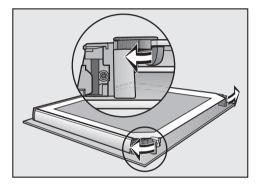
Flip the glass pane retainers outwards to open them. You can now remove the inner and the two middle panes.
