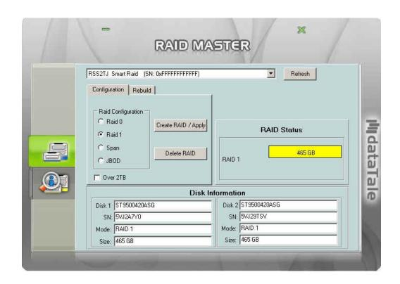
The Rebuild feature is only available under RAID 1 mode. If the "Rebuild" option tab is selected under any other RAID mode, a popup window will appear stating, "Attention! There should be two disks with at least one RAID 1 disk for Rebuild Mode."
