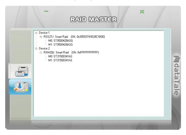
The connected RAID Unit(s) information with Device model of the RAID Unit(s), and serial numbers of each inserted HDDs.
