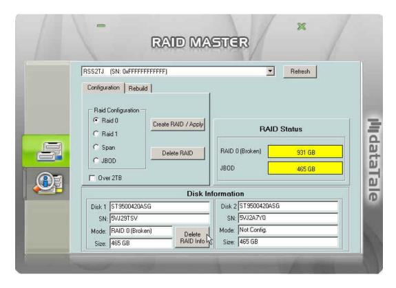
3. Once completed, the *New* HDD is ready to be used as JBOD or combined with the *existing* HDD under a chosen RAID mode.
