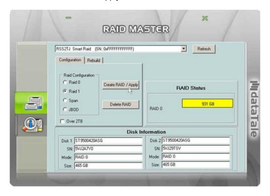
If the host can support more than 2TB HDD(s) storage capacities and the HDD(s) is/are over 2TB, remember to *check* the "Over 2TB" option under the "Configuration" option tab. Please see "Over 2TB" section under Q&As for more information. Please review the "DISK VOLUME OVER 2TB" section of the User's Manual for OS support information
