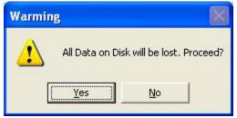
3. Once confirmed, the RAID MASTER will begin erasing the old RAID Mode for the chosen HDD(s). Once the process is completed, the "RAID Status" and "Disk Information" should reflect the chosen HDD(s) as JBOD (Non RAID). The chosen HDD(s) RAID is/are now ready to be used under the new preferred RAID Mode!
