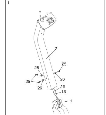
2. Connect the Reed Switch Wire (13) to the wire on the back of the Console (8).
