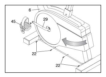
Remove the four #8 x 5/8" Screws (22) from the bottom of the Left Side Shield (6). Grasp both Side Shields at the top and gently pull them apart. Make sure that the arm of the Crank (29) is in the position shown in the drawing above. Hold the Left Side Shield at the rear and pull it gently away from the frame. Work the Left Side Shield forward off the arm of the Crank and remove it.
