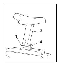
Insert the Lock Knob through one of the holes in the Seat Post and tighten it. **Do not insert the Lock Knob under the Seat Post.**
