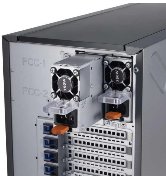
Figure 8. 750W power supply unit
