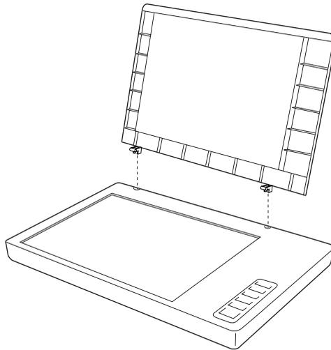
3. Make sure that the scanner is powered off; then plug the connector of the LightLid into the scanner's 9-pin accessory port.
