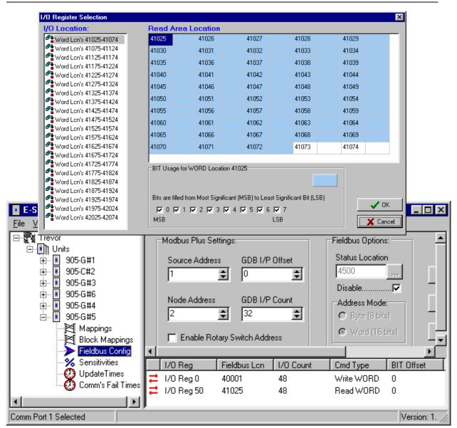
Finally, it must be taken into consideration that the 905G Modbus Plus module dynamically adjusts the 4X register range available to the network depending on the fieldbus mappings configured. The 905G will terminate the available 4X register range at the last mapped 4X register for both the read and write area. In the example above this means that the only 4X registers that are available to the Modbus Plus network are 40001 - 40048 and 41025 - 41072.
