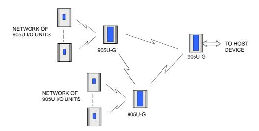
This type of network reduces the amount of radio traffic and is suitable for systems with a large number of I/O modules. The system is divided into local sub-networks, each with a 905G unit. The 905U modules transmit their I/O vlaues to the 905G. The 905G then transfers these values to the "central" 905G using a block transfer which is very efficient compared to a lot of individual I/O transmissions.
