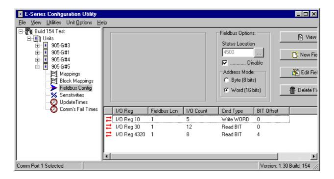
Three Fieldbus Mappings are illustrated in the example above. Note that "Word Address Mode" is selected, meaning that the Fieldbus Interface IN and OUT Areas will be treated as word-addressed arrays by configuration software. The parameters for each fieldbus mapping were setup using the mapping configuration screen as described above.
