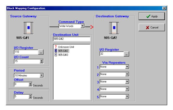
Select the "Command Type" from the pop-down window in the centre of the display. The red arrow will confirm the direction of the block transfer. Now select the destination module - only the 905G modules already configured will be shown. If you need to use repeaters in the radio link, enter the repeater addresses, starting with the repeater closest to the source module.
