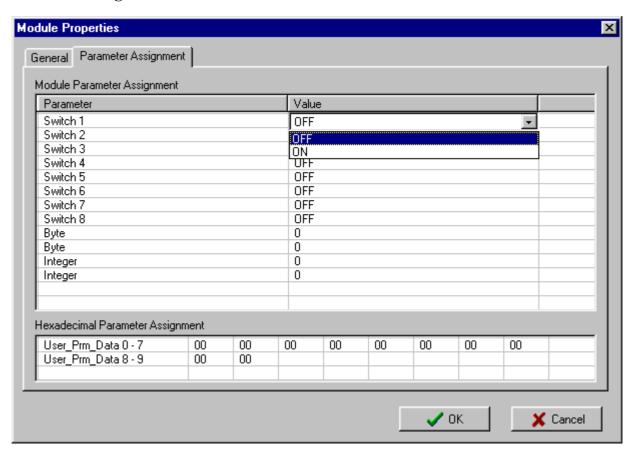
A slaves user-specific parameters can be changed via the *parameter assignment* page. User-specific parameters for a slave device are defined in the corresponding GSD file for the device, the definition of which are device-specific and should be found in the documentation for the device.
