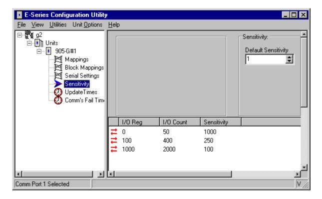
"Change" messages for both individual I/O mappings and block mappings use a sensitivity value to trigger the message. Sensitivities are configured for blocks of I/O registers - that is, each I/O register does not have a unique sensitivity. You can configure up to 50 sensitivity values - that is, there can be 50 blocks of registers with different sensitivities.
