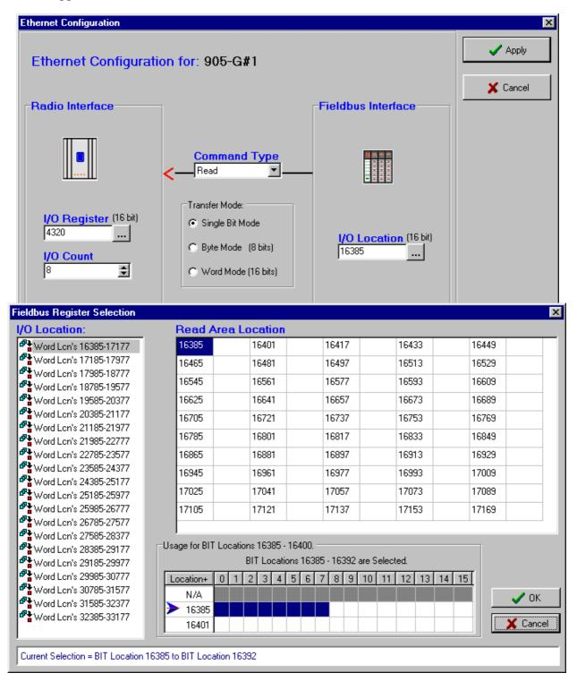
Appropriate Modbus prefixes may need to be added to the Modbus Address depending on the host device. For example, a "word write" fieldbus mapping in the 905G to Modbus location 10, can be read by a host device as 30010 (30000 for an input register + 10 as the address).
