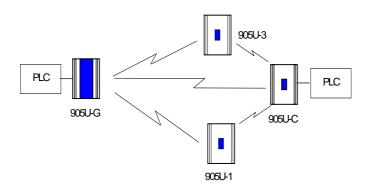
905G modules can transmit to 905G modules as well as other 905G modules. There can be multiple 905G and 905C modules in a network - as well as 905U I/O. Because the 905U protocol is peer-to-peer, there are few constraints on communications between multiple 905U modules.
