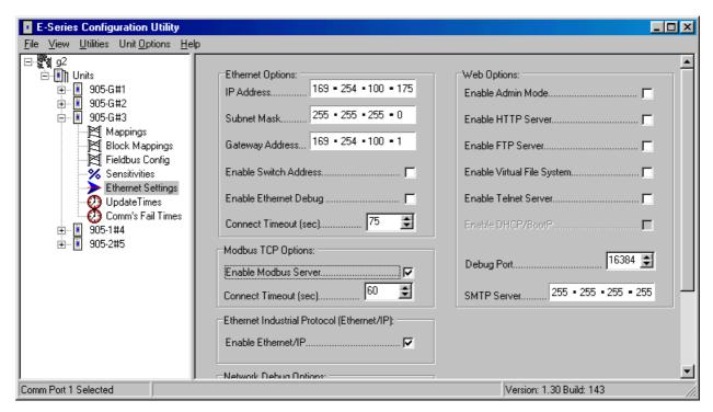
For example, a common subnet mask is shown in the example below. Looking at the IP Address located directly above the Subnet Mask in this example, it can be seen that the IP Address values directly above a subnet mask value of 255 correspond to the subnet ID. Conversely, the IP Address values directly above a subnet mask value of 0 correspond to the host ID. So, in this example, the subnet ID is 169.254.100 and the host ID is 175.
