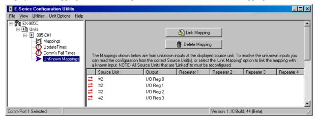
If you also load the configurations from the other remote modules in the system, then these unknown mappings will disappear as the program can determine where the remote inputs are. Alternately, you can select "Link Mapping" and manually enter the remote inputs.
