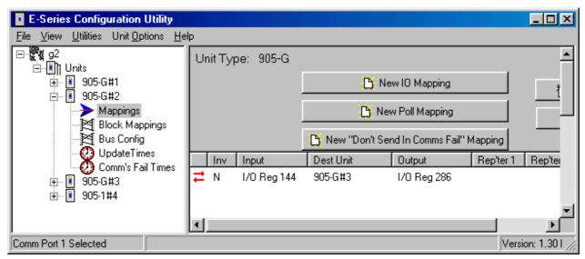
Whenever I/O Reg 144 changed by the sensitivity amount, 905G#2 would send a message to 905G#3 to write the value in I/O Reg 286. The problem arises if there are a lot of these mappings. Each radio message only relates to one register-register link. If you want to map 1000 registers from one 905G to another, then this could generate a lot of radio messages.
