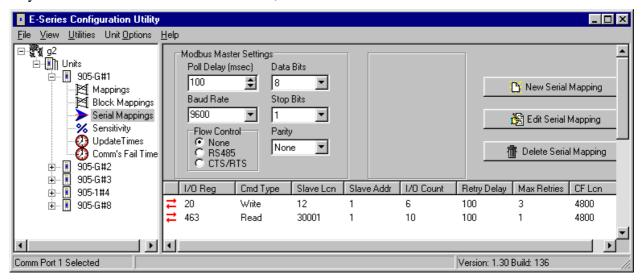
device/s. If the RS485 port is used, then multiple Modbus Slave devices can be connected to the 905G. The 905G Modbus Master will generate Modbus read and write commands to the Modbus Slave devices.
