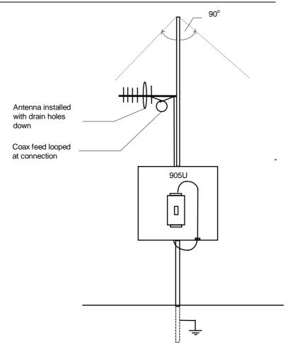
If there are more than two stations transmitting to a common station, then the Yagi antennas should have vertical polarization, and the common (or "central" station should have a collinear (non-directional) antenna.
