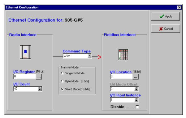
To make I/O data available via Ethernet/IP, ensure that the Enable Ethernet/IP checkbox on the Ethernet Settings page is checked. Appropriate Fieldbus Mappings need to be configured to link the required I/O registers to the Fieldbus Interface, as described above in the Profibus and Modbus/TCP sections. An "I/O Instance" for each fieldbus link must also be specified so that the configured I/O data is made available to one of the six possible Ethernet connections.
