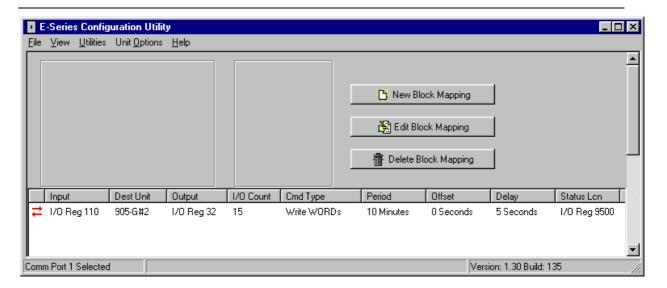
In the above example, the status register for the block mapping has been automatically assigned to register 9500.
