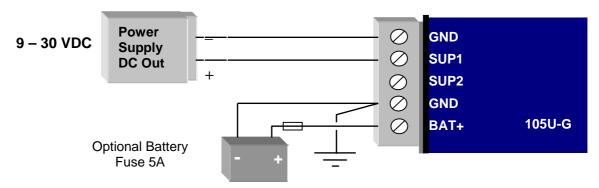
The module may also be powered from an external 11 - 15 VDC battery supply without the need for a "normal" supply connected to "SUP1". This external battery supply is connected to "BAT+" and "GND" terminals. The positive lead of the external supply should be
