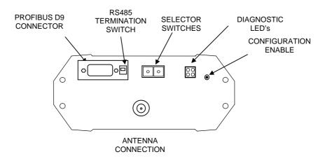
Note: If the "Use Rotary Switch Address" option in configuration software is selected, the two rotary switches are used to specify the Profibus Node Address in the range 0-99. In this case, the value on the left switch is multiplied by 10 and added to the value on the right switch to give the node address.
