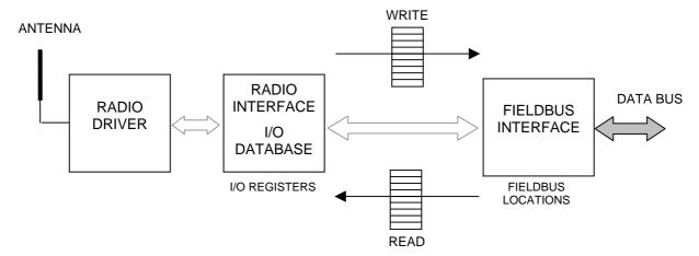
Software. The diagram shows in more detail the relationship between the Radio Interface and Fieldbus Interface.
