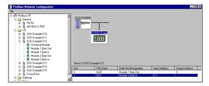
When these modules are added, configuration software automatically picks the next free *fieldbus interface* registers (shown in the *Input Address* and *Output Address* columns), which may later be altered by double-clicking on the relevant I/O module. In this example, the automatically chosen locations are *Fieldbus IN* locations 0..1, and *Fieldbus OUT* location 0.
