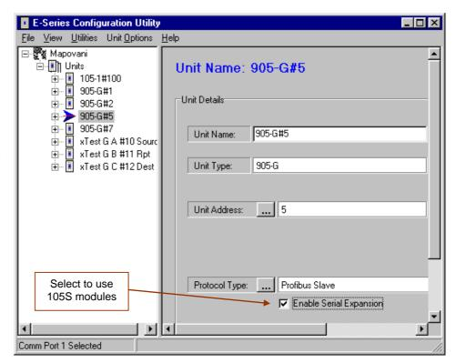
Note that enabling 105S expansion also disables on-line diagnostics via the serial port.
