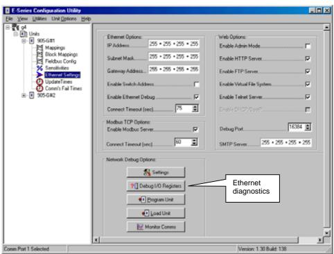
need to select 'Connect' under Debug Options. The Green / Red box will indicate the Connected / Disconnected State. Once connected select "Read" and check "Continuous". The display option allows you to view the registers in different formats, and you can select which I/O register you want to view from the left-hand side of the screen.
