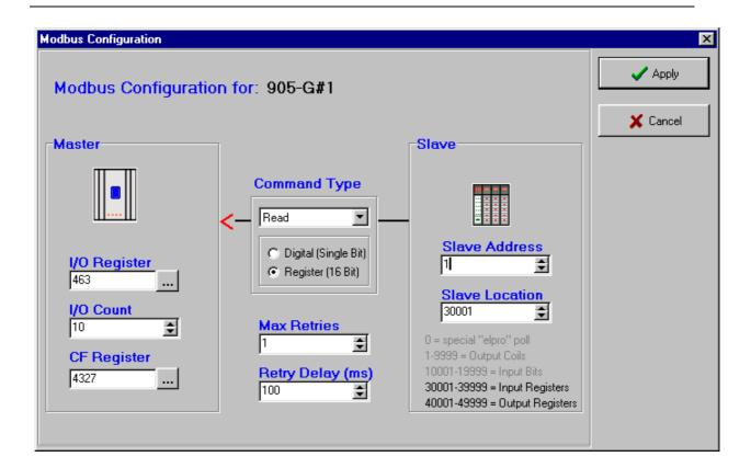
To complete the Fieldbus Configuration, enter any other Modbus commands that may be required to transfer I/O points between the 905G and the Modbus Slave devices.
