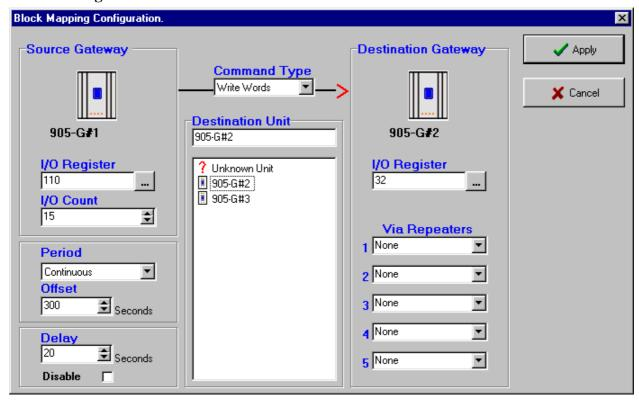
If a value in the block changes by more than the sensitivity amount, then the block message will be sent (this can only occur for Write mappings). The sensitivity values are set under the "Sensitivity" option as per section 4.5.
