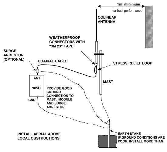
A collinear antenna transmits the same amount of radio power in all directions - it is easy to install and use. The dipole antenna with integral 15 ft (5m) cable does not require any additional coaxial cable, however the other collinear antennas do not have integral cable and an external cable length must be connected - such as the CC10 or CC20 cable kits..
