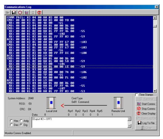
To decode the radio traffic using configuration software, first start communications logging by selecting option "c) Enable Comms Logging" from the debug menu. Next, in the diagnostics screen select 'Stop Terminal' and then 'Start Comms'. Configuration software
