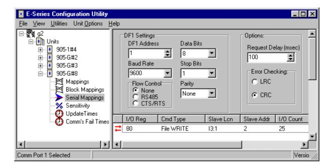
The entry under "I/O Register" (see below) is the first I/O register in the 905G to be transferred - the "I/O count" is the number of registers to be transferred.
