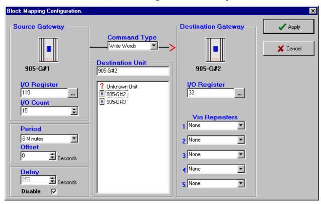
The "Offset" value provides an offset to the specified time. In this example, if the "Offset" was set to 10 seconds, then the messages will be sent 10 seconds later - at XX:00:10, XX:06:10, XX:12:10 etc.
