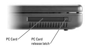
The computer recognizes most PC Cards and automatically loads the appropriate device driver. If the configuration program tells you to load the manufacturer's drivers, use the floppy disk or CD that came with the PC Card.
