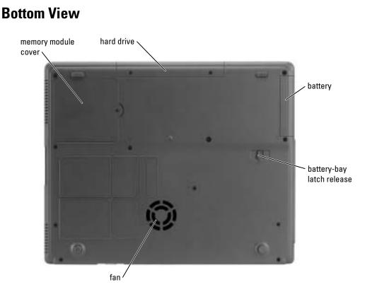
**MEMORY MODULE COVER** — Covers the compartment that contains the memory module(s).
