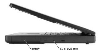
**BATTERY/BATTERY BAY** — When a battery is installed, you can use the computer without connecting the computer to an electrical outlet. See page 25.
