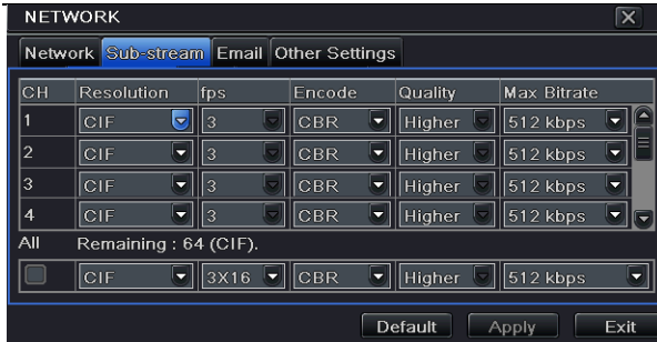
Fig 4-30 network configuration-sub stream
