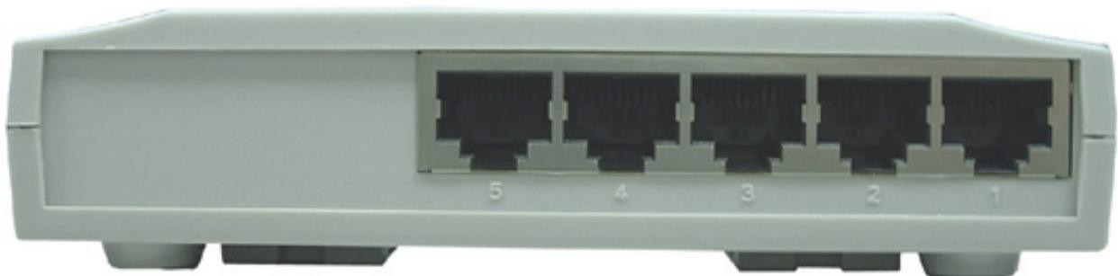
These jacks supports automatic MDI-II/MDI-X crossover detection function gives true ‘plug and play’ capability without the need of confusing crossover cables or crossover ports. Power is supplied through an external DC power adapter. Check the technical specification section for information about the DC power input voltage. Since the switch does not include a power switch, plugging its power adapter into a power outlet will immediately power it on.
