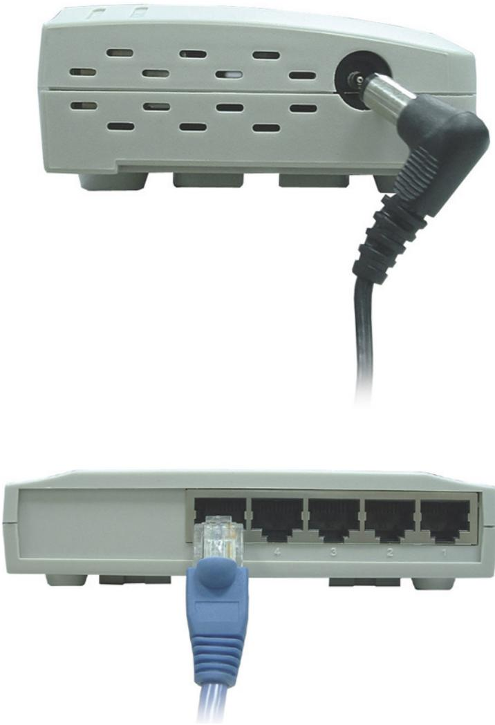
Power is supplied through an external DC power adapter. Check the technical specification section for information about the DC power input voltage. Since the switch does not include a power switch, plugging its power adapter into a power outlet will immediately power it on.
