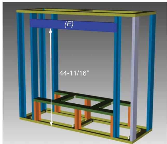
**12)** Line up screw holes on (E) (header) and (B) (inner vertical support). Secure with 2 wafer screws on each side (4 total) as shown below. This will now be the front of the frame.
