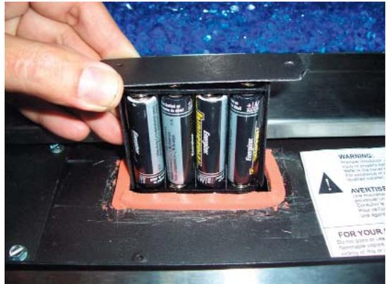
3) Install 4 - AA batteries and reverse steps.
