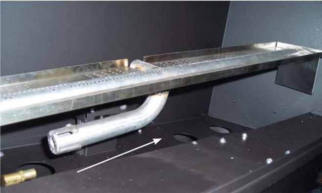
13) Remove the 5 screws securing the Digital Fireplace Burner Control to the firebox.
