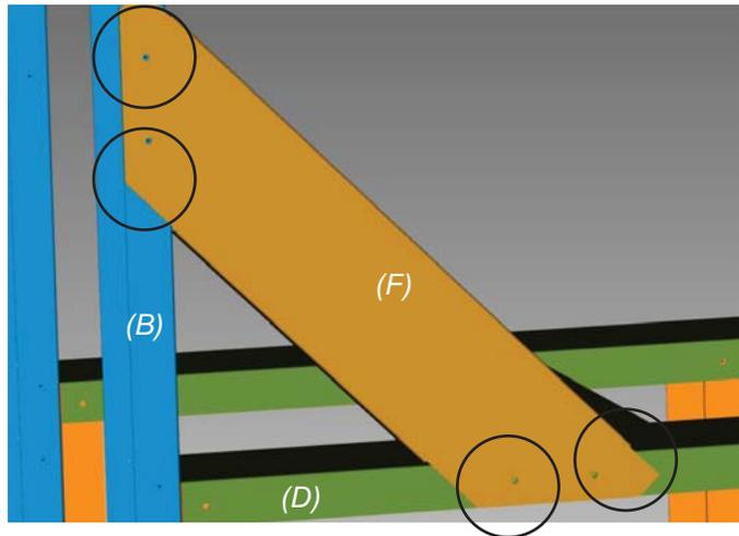
**16)** Install vertical back support to back of assembly with 2 screws at top and bottom in locations shown below.
