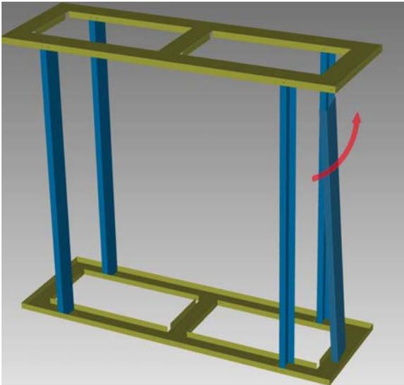
7) Line up screw holes on top / bottom (A) with each (B)- secure with 3 wafer screws each on top and bottom - 6 screws in total for each outer (B) (3 top- 3 bottom).
