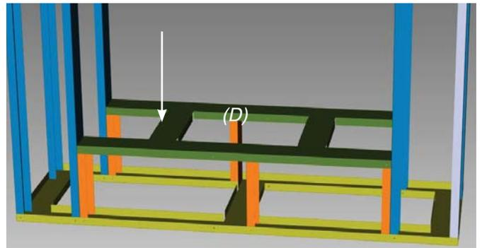
11) Measure 44-11/16" from floor (bottom of the header location) line up (E) (header) with appropriate screw holes.
