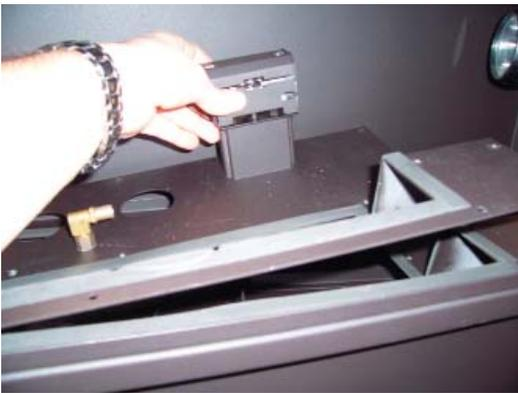
16) Replace with new valve tray and reverse steps. Inspect gasket condition, replace if necessary.
