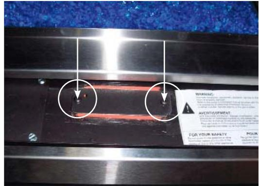
2) Lift the battery compartment upwards.
