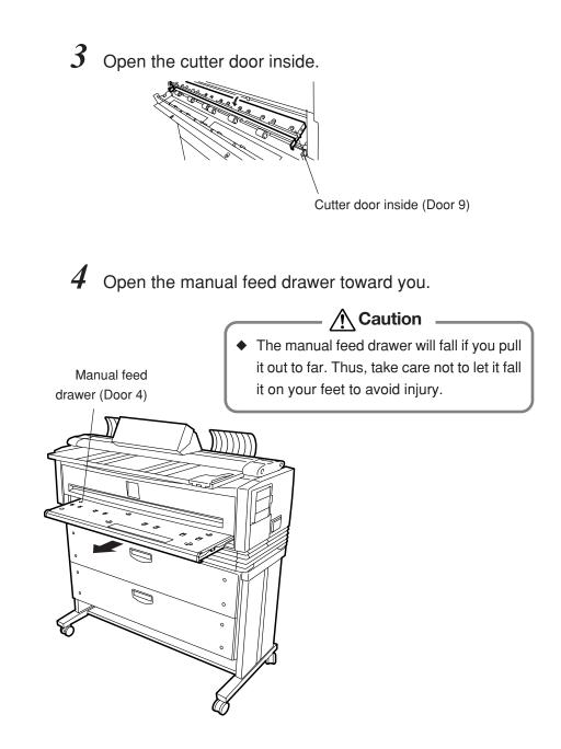
**5** Remove the jammed paper, insert the manual feed drawer and close the cutter door inside as well as the outside cutter door (door 5).
