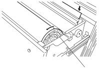
Turn the paper flange in the direction indicated in the illustration to such extent that the end of the wrinkled roll paper is visible.
