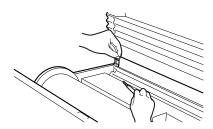
While holding the end of the paper roll, cut it with the cutter removing all of the wrinkled paper.
