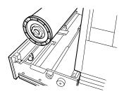
Hold the paper roll so that the end of the paper is positioned at the bottom facing the back of the device. Then align the paper flange to the depressions in the flange guide and gently insert the flange in place.
