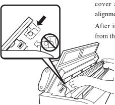
To insert the Process cartridge, align the Process cartridge with the angle of the open top cover and insert it in the direction of the alignment arrows (three points/green).
