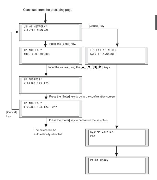
The device is "ONLINE" when it can receive and print data from the host computer and is "OFFLINE" when settings are being input on the control panel. You must set the device to "offline" to operate the menu from the control panel.
