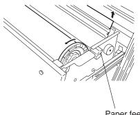
Turn the paper flange and insert the end of the paper roll so that it is straight. Turn the paper feed knob so that the end of the paper roll projects about 10 cm.
