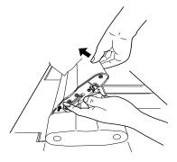
Lift the scanner cover up to its stop position. Pull the stopper towards the arrow direction and raise the scanner cover. The scanner cover will be held.
