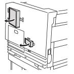
Pull out the filters toward you and remove, and replace with the two filters contained in the process cartridge packaging box.
