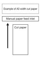
After the cut paper is properly fed into the manual paper feed inlet, the device pulls the paper into it.
