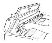
Pull the Process cartridge out by holding onto its handles.
