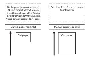
When plotting at the actual length or expanded size of a fixed form, load the paper as shown below (paper should be always set lengthways).
