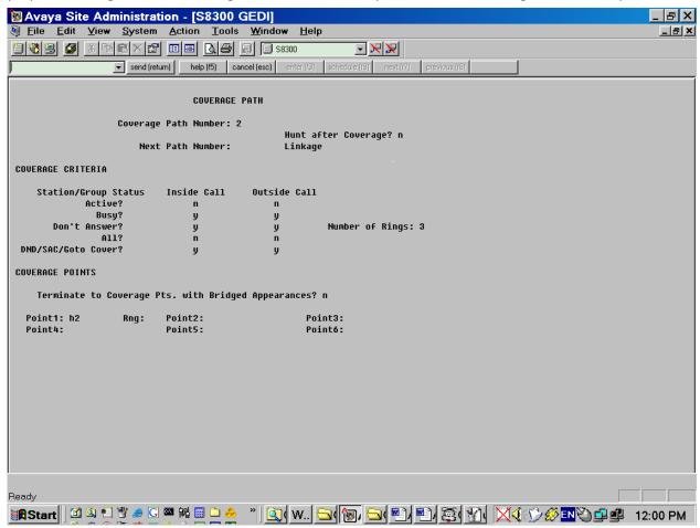
The coverage path example configured in the figure above, means that when the station does not answer the call or the call is busy, the call is forwarded to hunt group 2 (Point1: h2).
