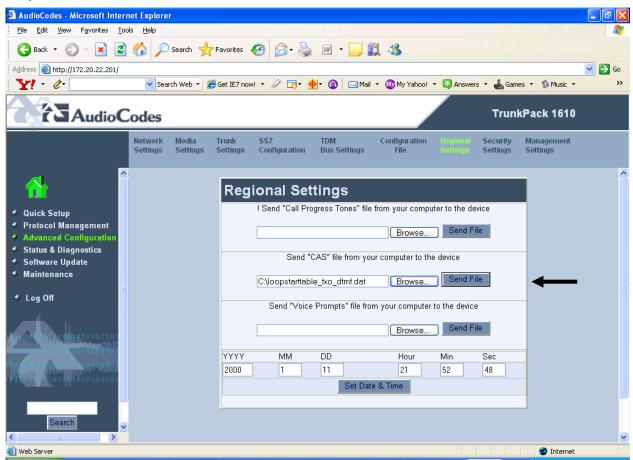
**Note:** The CAS file must be downloaded to the Mediant 2000. A suitable CAS file is attached to this document (refer to Section 4.1).
