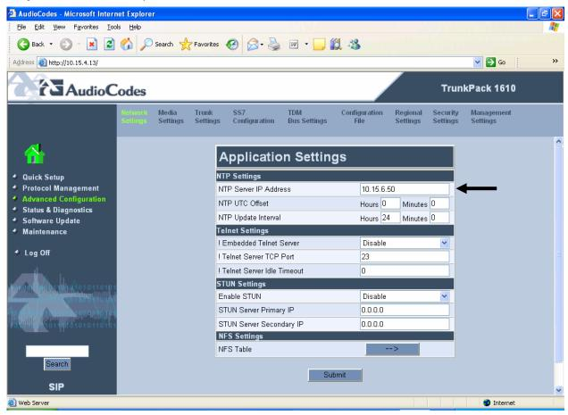
**Note:** Define the NTP server's IP address so that it corresponds to your network environment (for example, 10.15.3.50). If no NTP server is available in the network, then skip this step (as the gateway uses it's internal clock).
