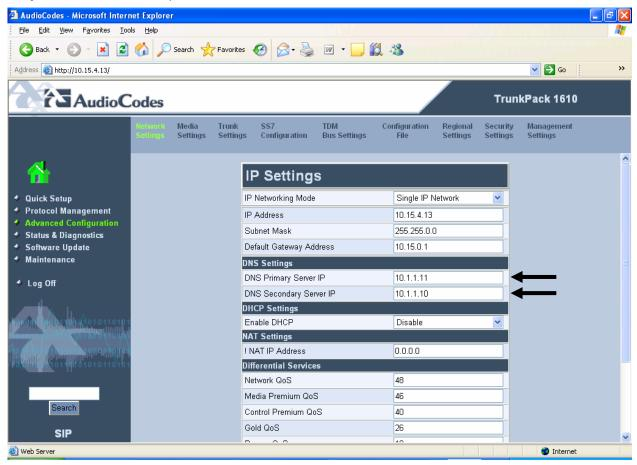
**Note:** Define the primary and secondary DNS servers' IP addresses so that they correspond to your network environment (for example, 10.1.1.11 and 10.1.1.10). If no DNS server is available in the network, then skip this step.
