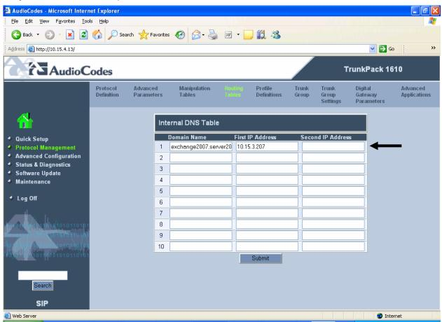
**Note:** If no DNS server is available in the network, define the internal DNS table where the domain name is the FQDN of the Microsoft Unified Messaging server and the First IP Address corresponds to its IP address (for example, exchange2007.com and 10.15.3.207).
