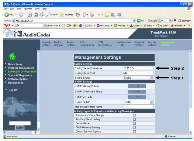
**Note:** The Syslog Server IP address must be one that corresponds to your network environment in which the Syslog server is installed (for example, 10.15.2.5).
