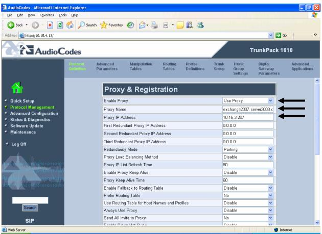
**Note:** The Proxy IP Address and Name must be one that corresponds to the network environment in which the Microsoft Unified Messaging server is installed (For example, 10.15.3.207 for IP Address and exchange 2007. server 2003. com for the FQDN of the Microsoft Unified Messaging host).
