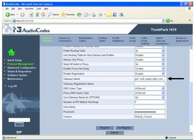
**Note:** Assign an FQDN name to the gateway (for example, gw1.m2k.audiocodes.com). Any gateway name that corresponds to your network environment is applicable; the only limitation is not to include underscores in the name (Windows Certification server limitation).
