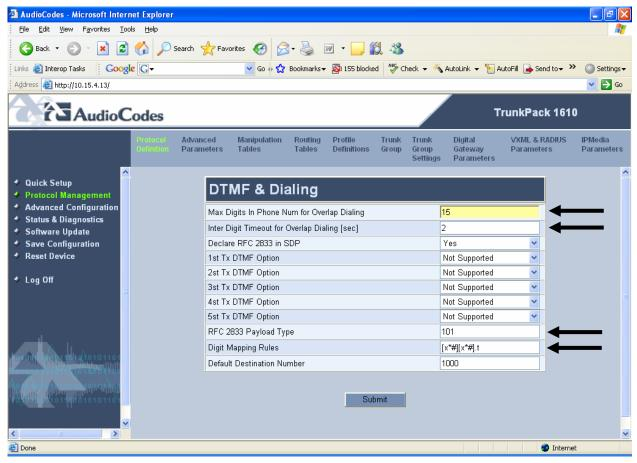
Step 5: Manipulation Routing Setup
