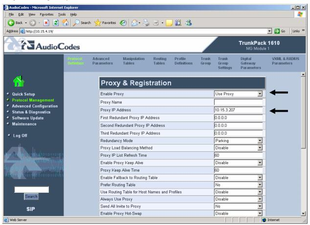
**Note:** The Proxy IP Address must be one that corresponds to the network environment in which the Microsoft Unified Messaging server is installed (For example, 10.15.3.207 or the FQDN of the Microsoft Unified Messaging host).
