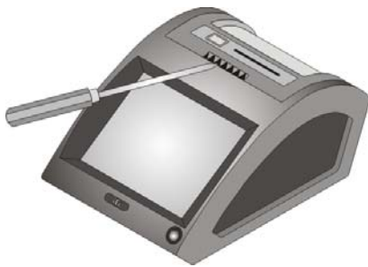
Figure 2-16: Push the Paper Cutter into Place
