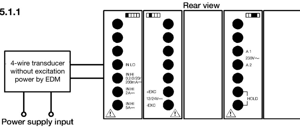
If the instrument has to be connected to 4-wire transducers, connect to screw terminals as shown in the figure.
