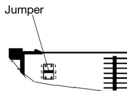
For voltmeters, ammeters, ohmmeters, frequency - and tachometers a jumper in the module determines the actual range for the module. Switching from one range to another also means that you are switching from one input circuit to another input circuit.
