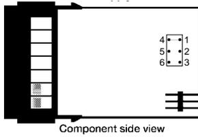
Range determined by jumper only. No software programming necessary.
