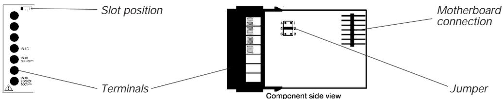
All modules are easy to plug in - for your information the slot position is marked on the drawing on the rear of the module.
