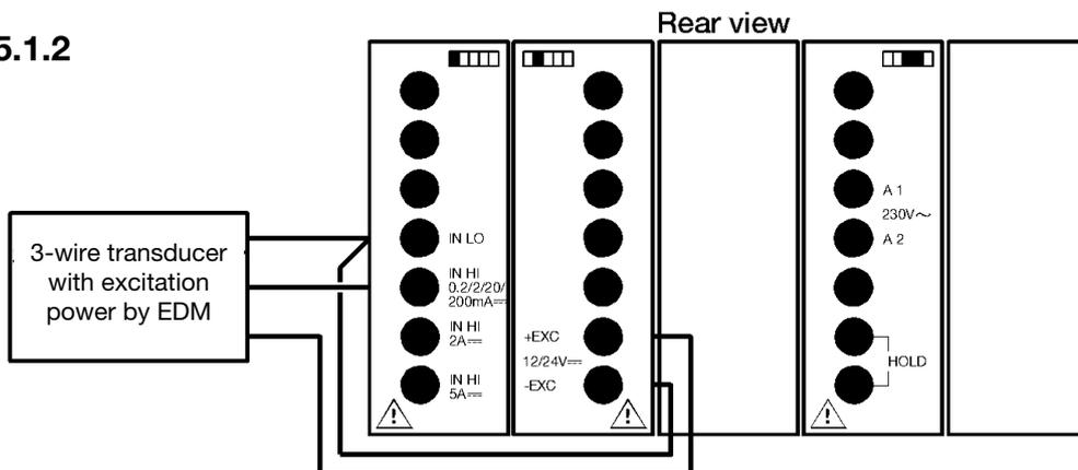
If the instrument has to be connected to 3-wire transducers powered by the instrument, connect to screw terminals as indicated.
