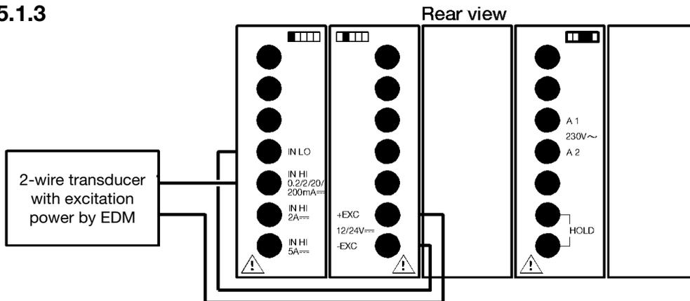
Connect as indicated if the instrument has to be connected to 2-wire transducers powered by the instrument.
