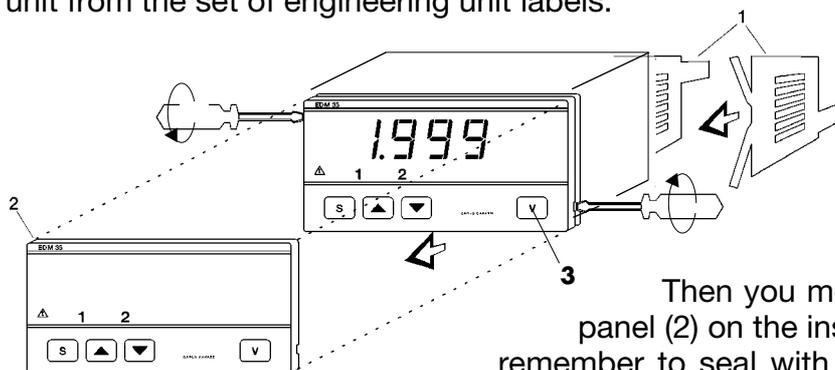
Then you mount the front panel (2) on the instrument - remember to seal with the enclosed gasket (the largest of the two enclosed). Place the remaining gasket round the body of the instrument and slide instrument into the panel aperture. **To optimize the tightness be sure that the panel cut-out is completed and deburred. Be also aware that a too thin panel may distort and not provide sufficient sealing.**
