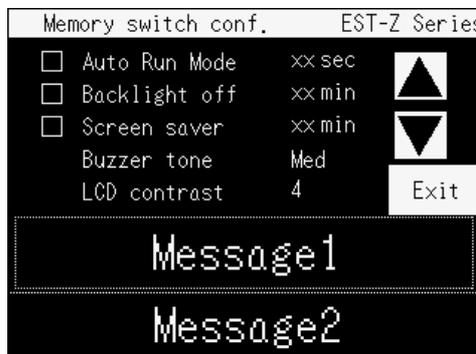
To activate Auto Run Mode, Backlight off, and Screen saver, touch  on the left. An activated item will be indicated with .
