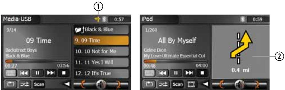
1. Once you have started a route guidance in the navigation mode you can change to an audio source that is supported by the splitscreen mode, by touching the [
