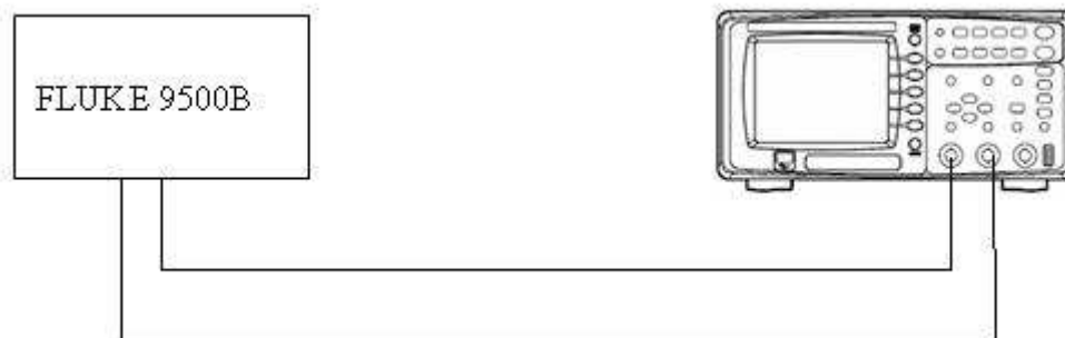
Picture 3-9 Test instrument connecting
