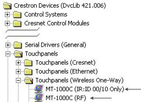
The system tree of the control system displays the device in the appropriate slot(s) with a default RF ID or IR ID as shown in the following illustration.
