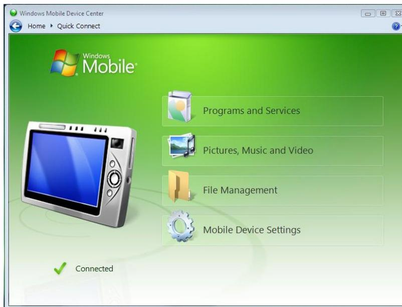
11. Toolbox can only see the MT-1000 if the Mobile Device Center looks like the figure above. If it does not, try reinserting the USB connector and reinstalling the driver.
