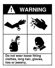
Follow good machine shop practices. Rotating shafts and components can entangle and enwrap, and can result in serious injures. Never wear long hair, loose-fitting clothes, gloves, ties, or jewelry when working with or near a drill or any machine with exposed rotating shaft.
