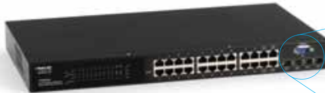
LPB4024A with (4) dual-media ports, each with (4) RJ-45 shared SFP ports. Dual-media ports can be used as either an extra copper 10/100/1000 PoE port or for adding a 1000-Mbps fiber uplink (optional SFP required).
